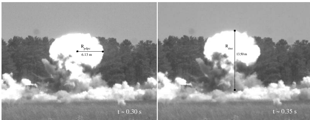
Figure 10. Fireball from event E7 at: (a) t = 0.30 s with a fireball radius of 6.13 meters and (b) at t = 0.35 s, with a rise relative to the blast origin of 13.5 m.
