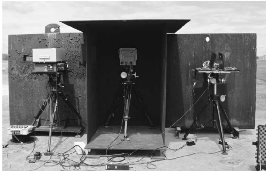
Figure 2: Left to right, the ABB-Bomem MR-254 FTS, CI Systems ColoRad radiometer, and pair of Phantom 5.1 and 7.1 cameras. Each is peering through a hole from behind thick iron armor shielding. A plywood roof was subsequently installed to shield the instruments from heating via direct sunlight, thereby minimizing the effects of self-emission in the InSb channel of the FTS and the InSb and HgCdTe channels of the radiometer.
