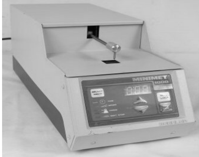
Figure 9. The Buehler MiniMet 1000 was used to remove \text{SiO}_2 from the backside of many PLD samples.
