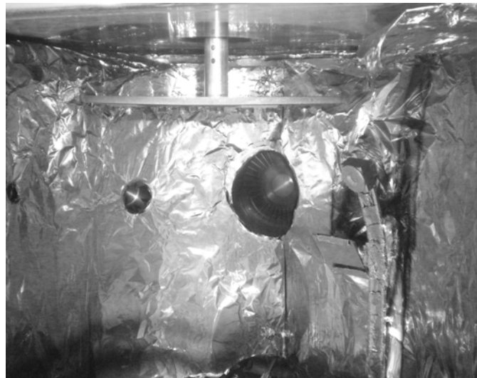
Figure 15. The chamber attachment was affixed to a rotating metal dowel in the top part of the chamber. The attachment rotated inside the chamber to provide a uniform distribution of metal on the sample.
