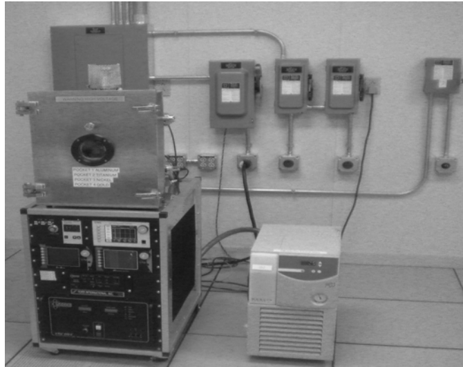
Figure 11. The electron beam evaporator was used for most metalizations to apply both front and back contacts on the samples. The picture shows the chamber, controls, and pumps.
