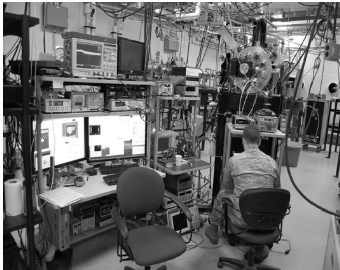
Figure 31. The measurement setup utilized a laptop, CV meter, and a voltage source. Cables were fed from the CV meter to the outside of the irradiation chamber. The QASPR III controls were many and elaborate, however in house Labview programs controlled the beam and an oscilloscope verified the current in the beam line.
