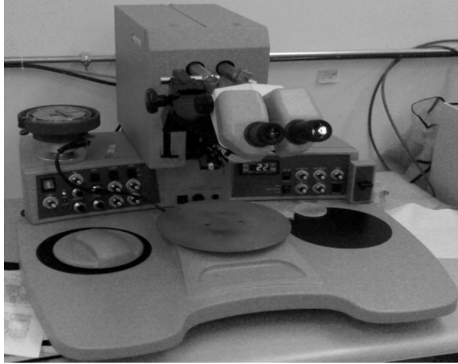
Figure 17. A Kulicke and Soffa Model 4526 Analog Ultrasonic Compression Wedge Wire Bonder was used to affix 0.0007" diameter wire to the top circular contacts of the samples.
