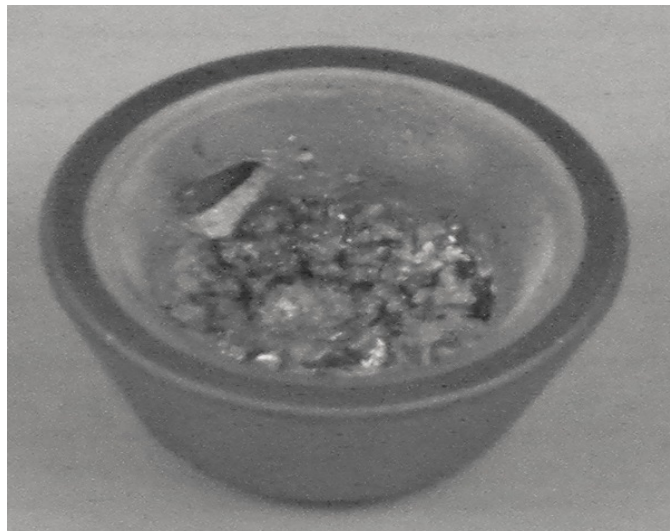
Figure 12. A copper crucible held a cylindrical pellet of the contact metal. An electron beam evaporated the metal from inside the crucible.
