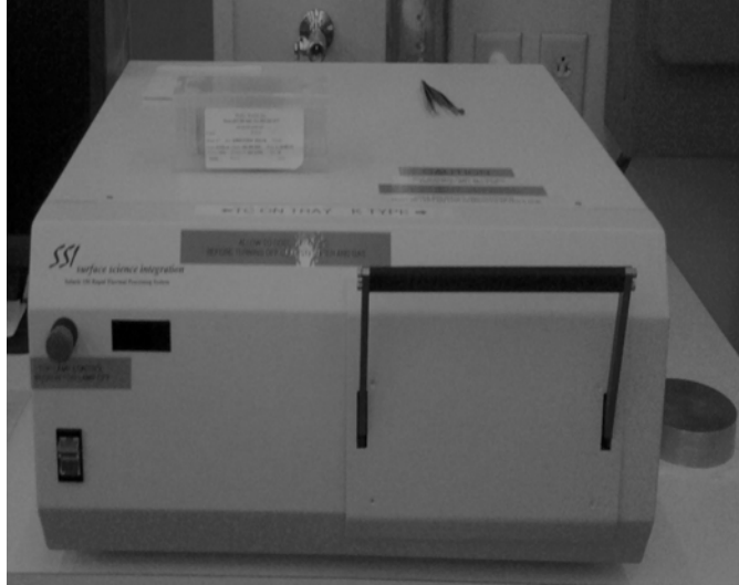
Figure 16. Selected PLD samples were annealed by heating them to 450°C for 30 seconds. Samples sat loosely on a 3 inch diameter silicon wafer inside the chamber.
