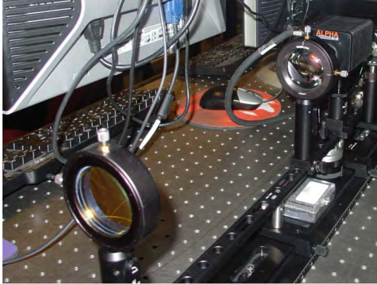
Figure 25. Imaging system showing the 300mm lens and the 75mm lens followed by the FLIR Alpha NIR camera.
