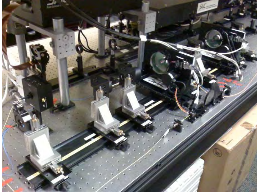
Figure 26. Atmospheric Turbulence Simulator.
