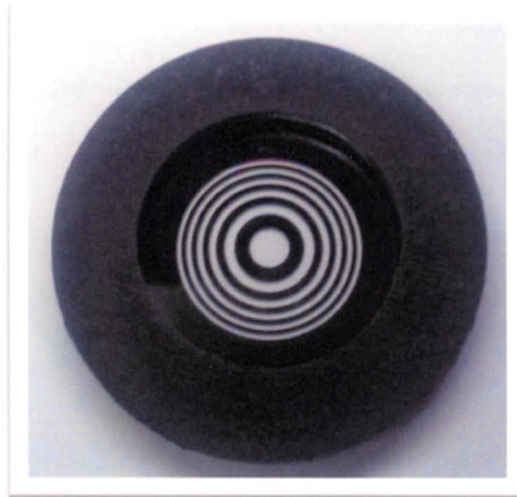
Figure 1-2 Fresnel Zone Plate Aperture as Coded Aperture
