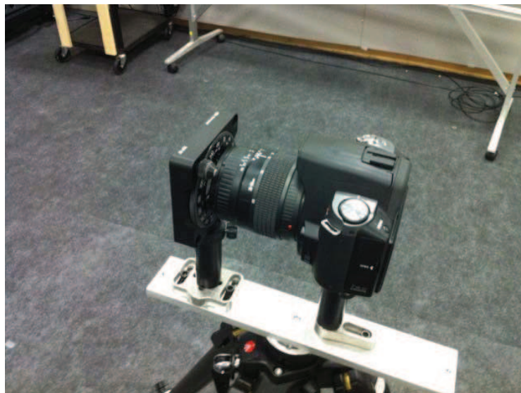
Figure 3.7: Physical System Setup. A visible Sony CCD camera mounted behind a linear polarizer in a rotation stage.
