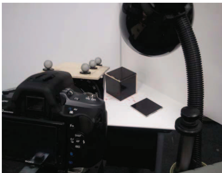
Figure 4.22: Camera orientation test setup in the Vicon lab. This image shows the camera, the light source, reflection panels and the glossy black cube test subject.
