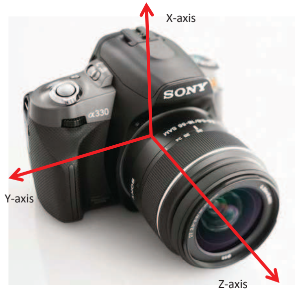
Figure 2.1: Common coordinate system for a camera reference frame. This figure shows the x -axis pointed out the top of the camera, the y -axis pointed out the right hand side and the z -axis pointed out the front of the camera from the center of focus through the optical center of the lens.
