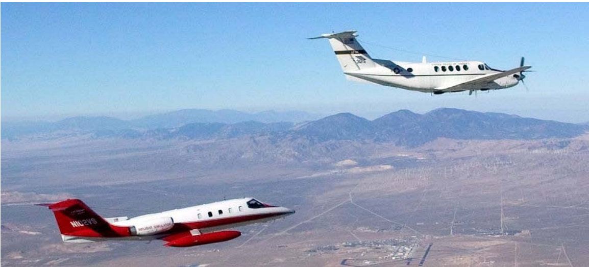
Figure 4.1: Differential GPS AAR between a C-12 and a LJ-24 [16]. This successful demonstration proved the capability of AAR and led to many future projects.
