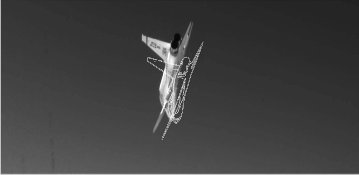
Figure 5.13: Time sync maneuver. Four different data sources were synced together using a few time sync maneuvers through the flight. The contour overlay is from the combination of the two GAINR unit's truth data. A position bias between aircraft in the truth data is visible by the non-intentional offset.
