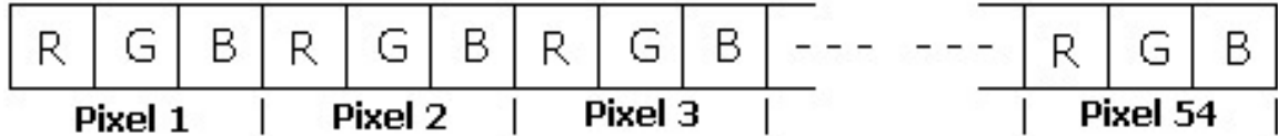
Figure 2.23: OpenGL image storage configuration [1]. OpenGL accesses pixel information from an image using a single array with a length equal to the total number of image pixels \times three.
