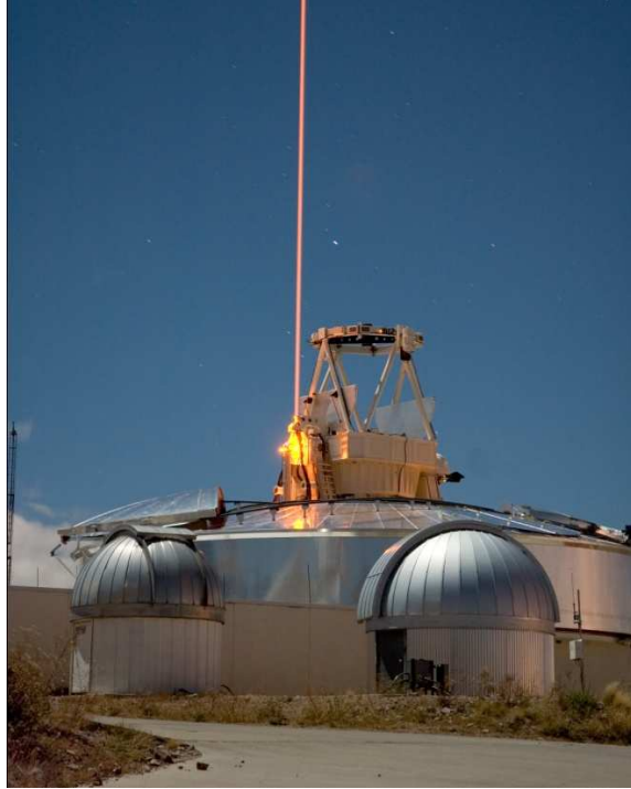
Figure 11. The 3.5 meter telescope at SOR. This long exposure photo shows the exposed telescope aperture and the sodium LGS.
