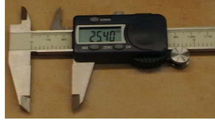
(b) Digital caliper for measuring distances
