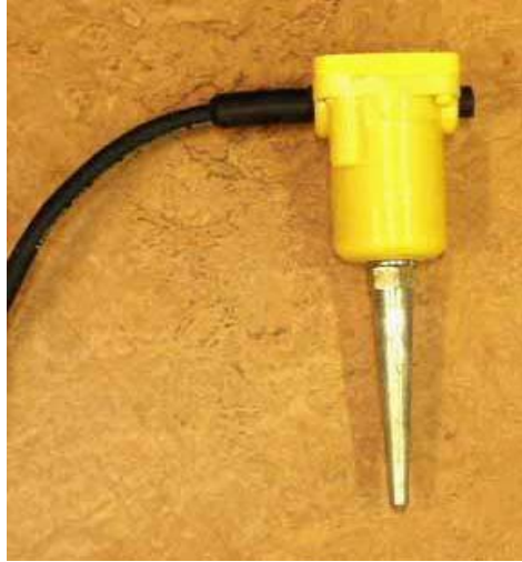
Figure 4: SM6-U/B Geophone, taken from Lindgren, Habberstad, and Holmberg [16]
