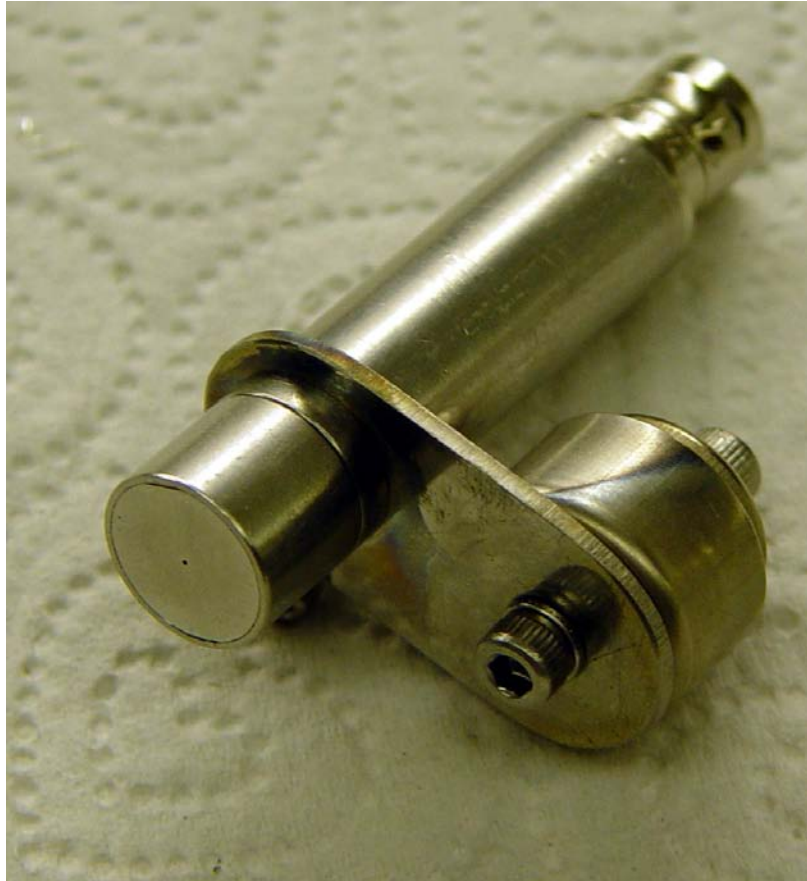
Figure 25: Photo of Faraday probe, taken from Faraday Probe Operating Manual [64].
