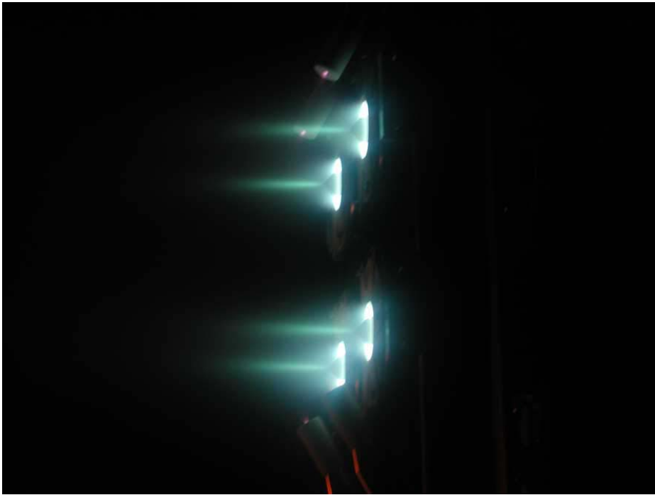
Figure 10: A cluster of four BHT-200 thrusters in operation [47].
