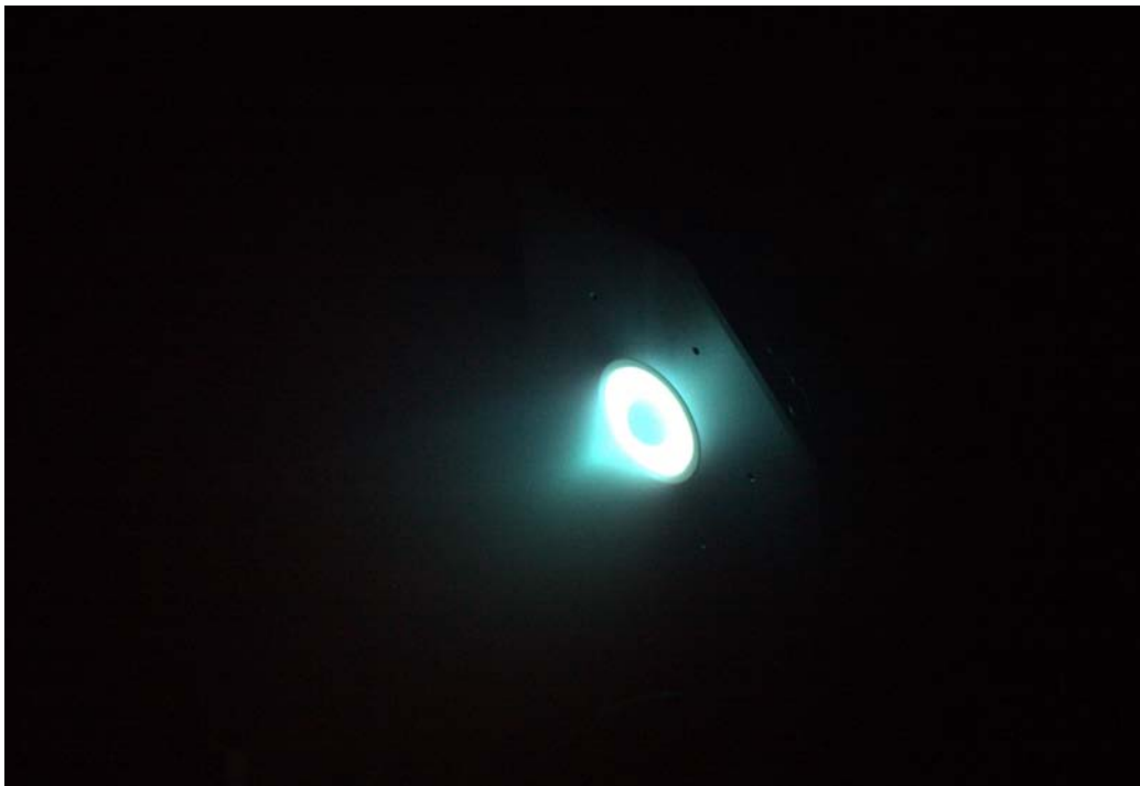
Figure 32: X-face of thruster displaying ball plume mode.
