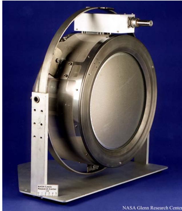
Figure 2: NASA NSTAR ion thruster, from NASA Glenn Research Center [5].
