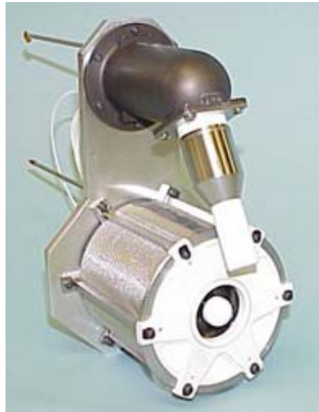
Figure 18: BHT-200 thruster with BHC-1500 cathode on mounting bracket [60].
