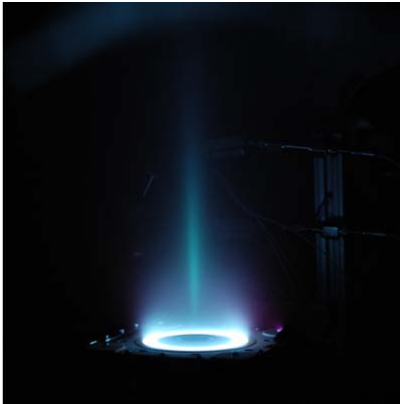
Figure 8: Visible plasma plume of BHC-1500 Hall effect thruster during ground testing.
