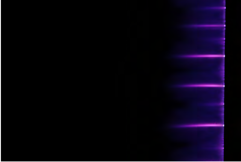
Figure 2.8: 1.8mm thick silica dielectric based sliding discharge actuator at its saturation potential of 19 kV.
