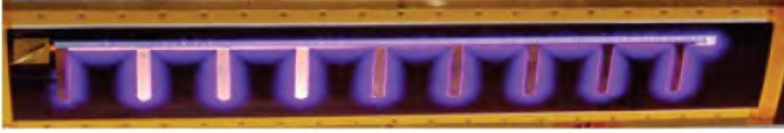
Figure 1.2: Chordwise arrayed DBD actuators increase the span wise effective area of the DBD plasma. From Poggie et. al. [22]
