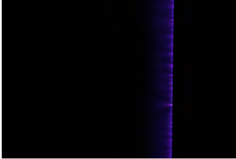
(a) Glow discharge as seen with a 30 Hz shutter speed for a 15 kV potential DBD.
