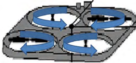
Figure 40. Quadrotor Opposing Pitch Propellers
