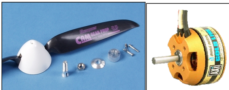
Figure 29. Propeller (left) and motor (right) of the GenMAV 2
