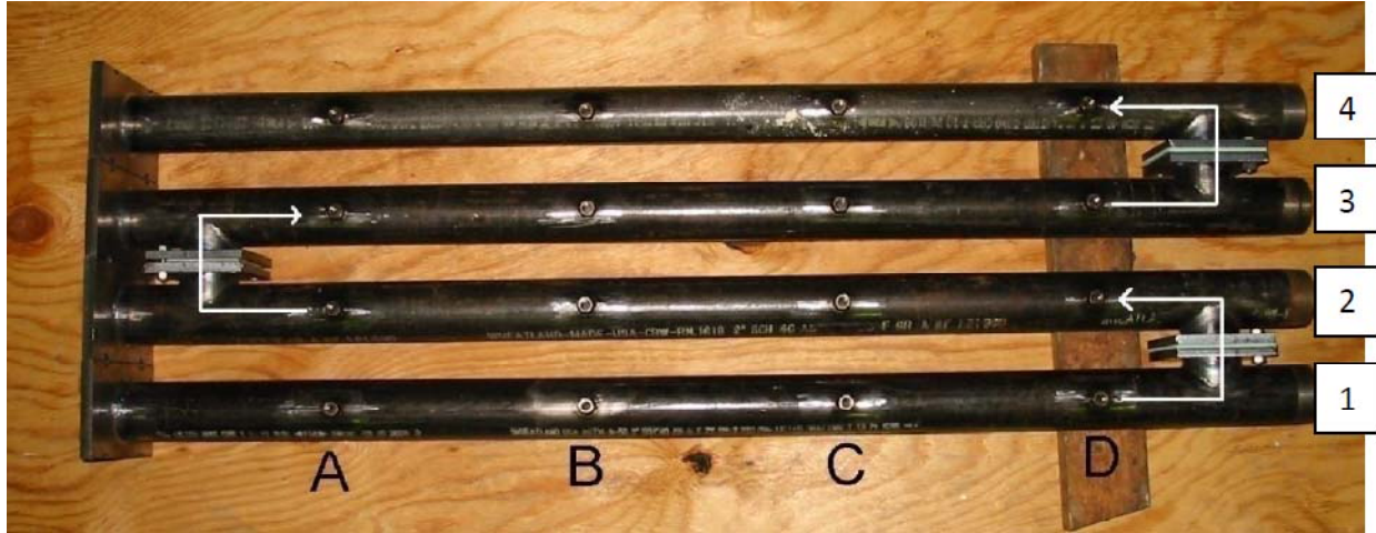
Figure 4. Four-tube setup successfully run on ethylene and hydrogen using tube-to-tube initiation. Arrows show direction of detonation wave.
