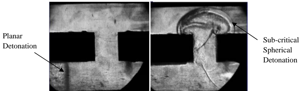
Figure 13. Representation of a planar (left) and a sub-critical spherical detonation (right). Propagation for the planar detonation is left to right in the bottom tube. Propagation for the sub-critical spherical detonation is bottom to top.
