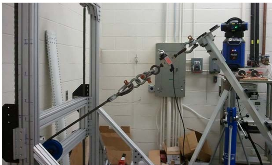
Figure 3.2: Qualification Model under a Follower-Force Load
