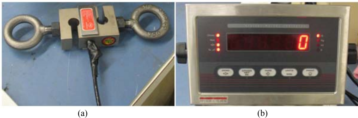
Figure 3.10: Load Measuring Instruments (a) Load Cell and (b) Weight Indicator
