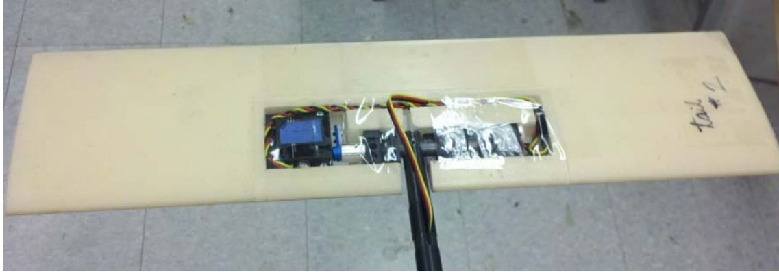
Figure 57. Completed Elevon/Servo Assembly
