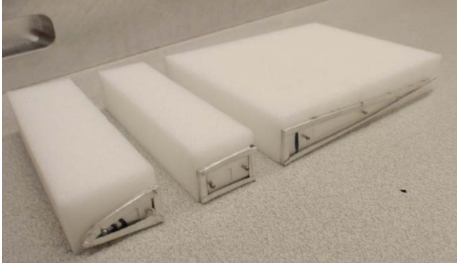
Figure 26. Rohacell 31-IG Foam Airfoil Guides [25]
