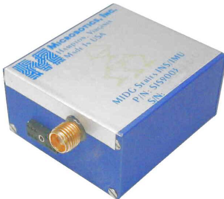
Figure 65. The MIDG II GPS/INS
