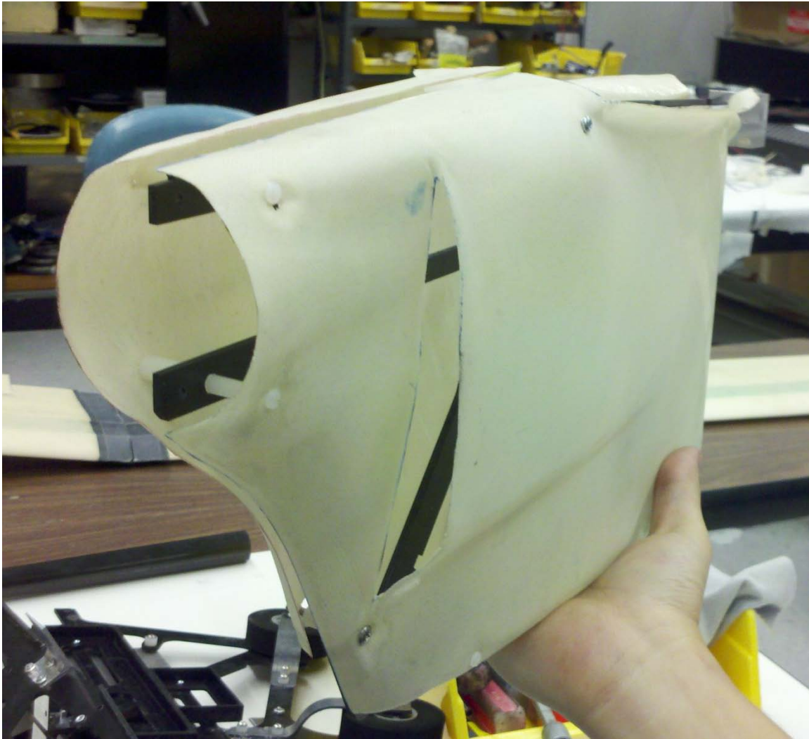
Figure 50. Completed Fairing Shell with Carbon Spine
