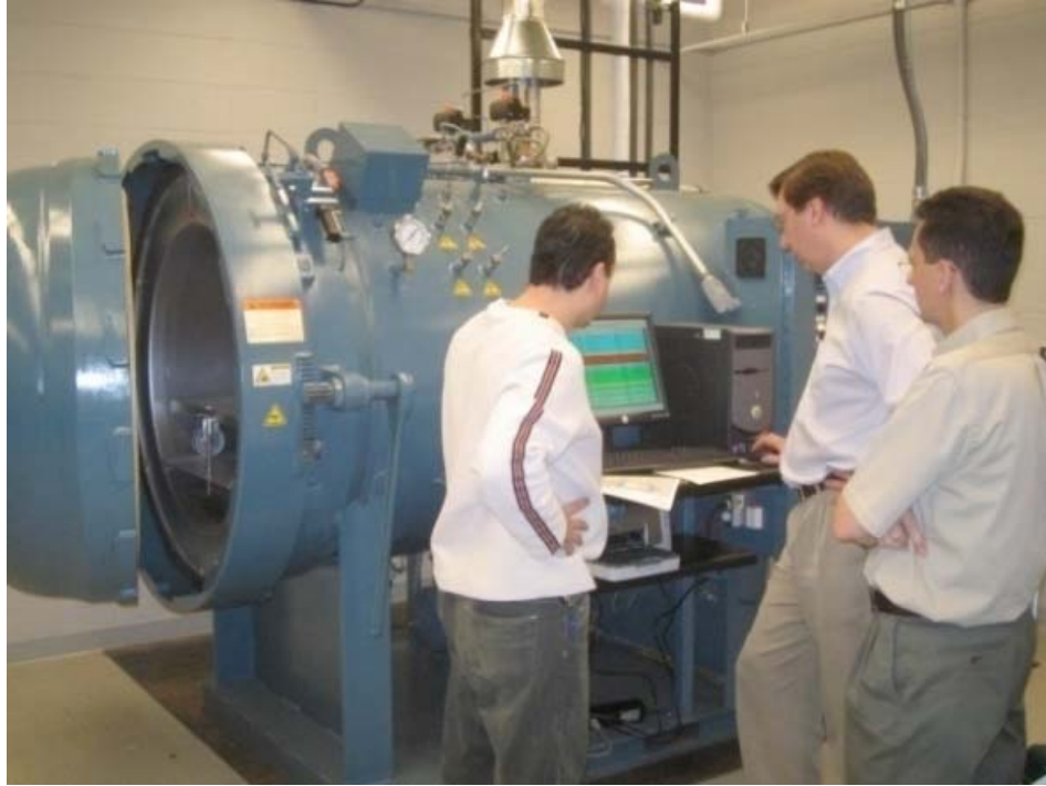
Figure 36. The University of Michigan's Engineering Autoclave [5]
