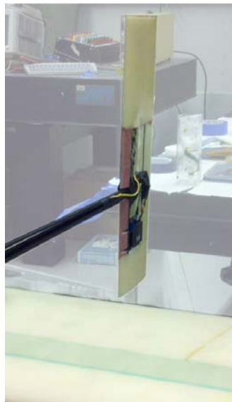
Figure 61. Built Vertical/Horizontal Tail in Vertical Position
