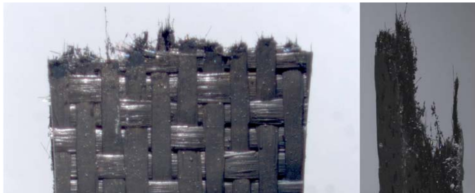
Figure 36: Optical micrographs of specimen P7-7 tested in tension at 1200°C in air. UTS = 406.9 MPa.
