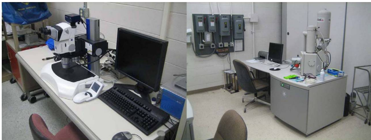
Figure 9: Zeiss Stemi SV II optical microscope (left) and Quanta 200 scanning electron microscope (right).
