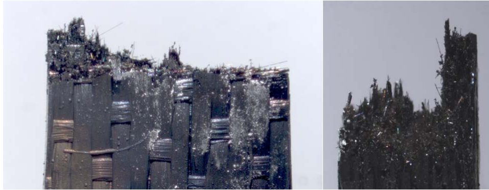
Figure 35: Optical micrographs of specimen P5-7 tested in tension at 1200°C in air. UTS = 296.3 MPa.
