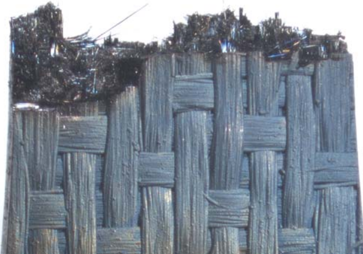
Figure 59: Optical micrographs of specimen P7-1 tested in fatigue at 1200°C in air. \sigma = 160 MPa, N_f = 6914 .
