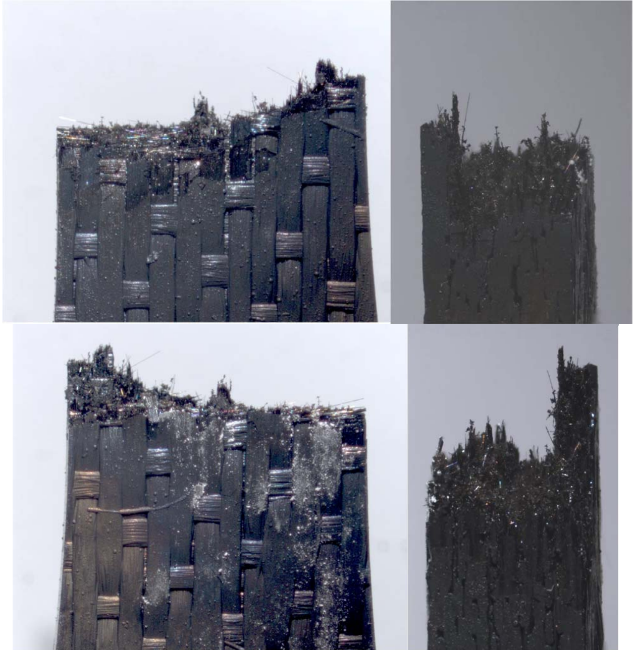
Figure 58: Optical micrographs of specimen P5-7 tested in tension at 1200°C in air. UTS = 296.3 MPa.
