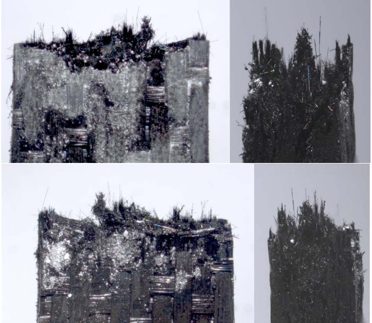
Figure 62: Optical micrographs of specimen P7-7 tested in tension at 1200°C in air. UTS = 406.9 MPa.
