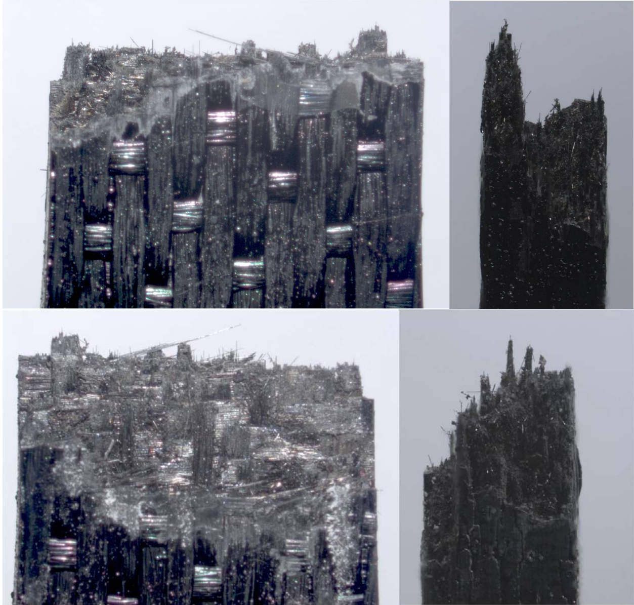
Figure 57: Optical micrographs of specimen P5-4 tested in fatigue at 1200°C in steam. \sigma = 140 MPa, N_f = 12784 .
