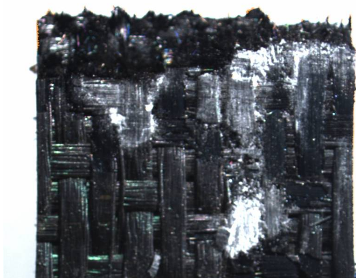
Figure 68: Optical micrographs of specimen P10-6 tested in fatigue at 1200°C in air. \sigma = 80 MPa, N_f = 200000 .
