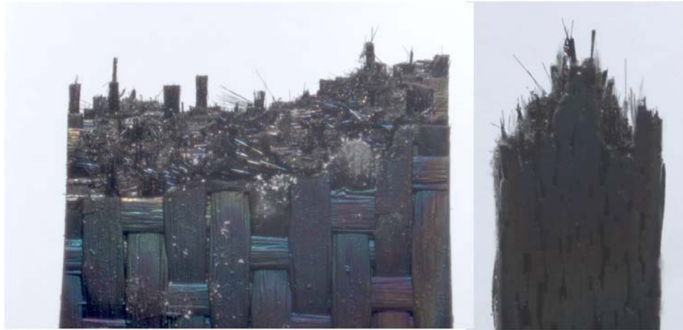
Figure 41: Optical micrograph of specimen P7-4 tested in fatigue at 1200°C in steam. \sigma = 200 MPa, N_f = 948 .
