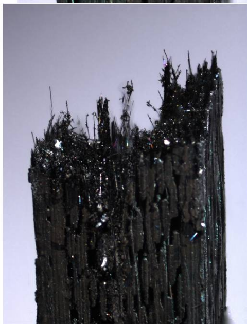
Figure 68: Optical micrographs of specimen P10-6 tested in fatigue at 1200°C in air. \sigma = 80 MPa, N_f = 200000 .
