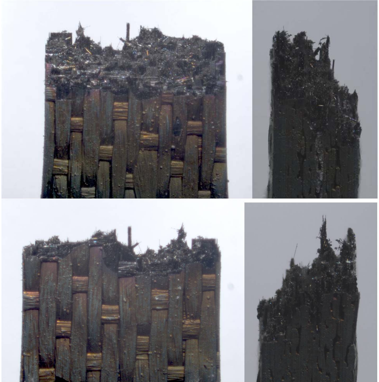
Figure 56: Optical micrographs of specimen P5-3 tested in fatigue at 1200°C in air. \sigma = 160 MPa, N_f = 29988 .
