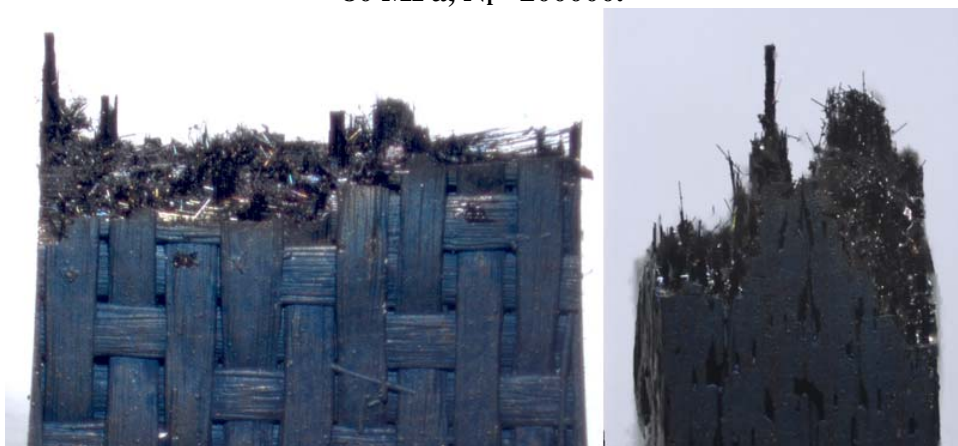
Figure 39: Optical micrograph of specimen P5-2 tested in fatigue at 1200°C in steam. \sigma = 80 MPa, N_f = 200000 .
