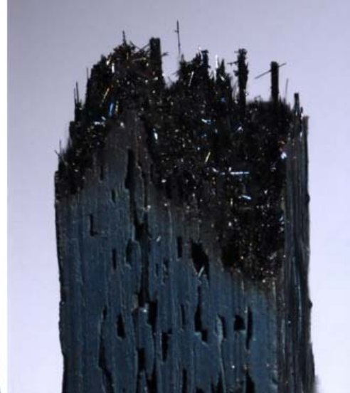
Figure 59: Optical micrographs of specimen P7-1 tested in fatigue at 1200°C in air. \sigma = 160 MPa, N_f = 6914 .
