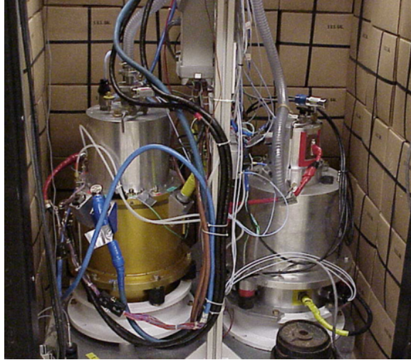
Figure 1: Photo of NASA's D1 and HSS flywheels demonstrating integrated power and attitude control, July 2003 (19:64)
