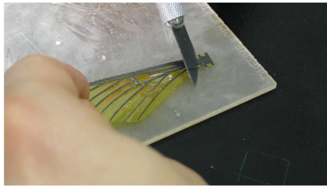
(e) Construction Vein Removal
