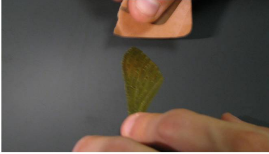
(a) Sanding of Completed Wing
