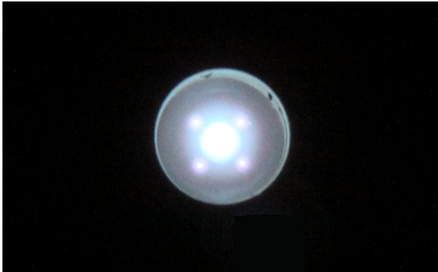
Figure 3. Thruster discharge channel during low power operation.
