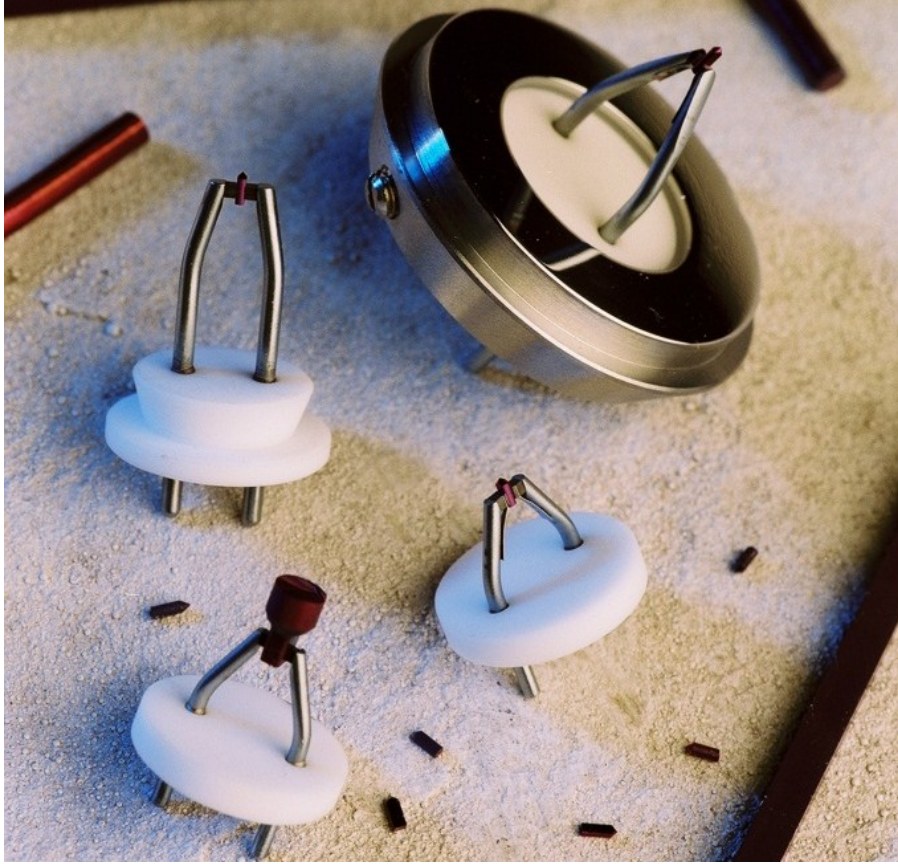
Figure 9. Depiction of multiple Lanthanum Hexaboride crystal emitter designs, used with permission of Applied Physics Technologies.
