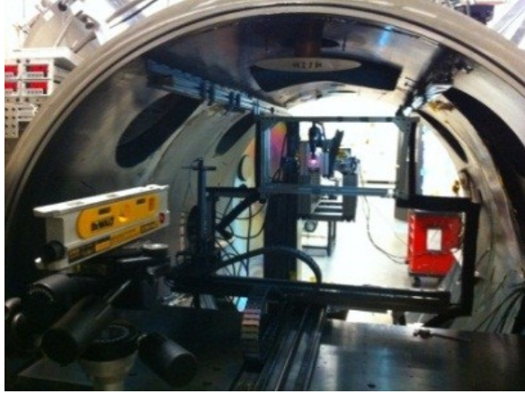
a) Laser level positioned.
