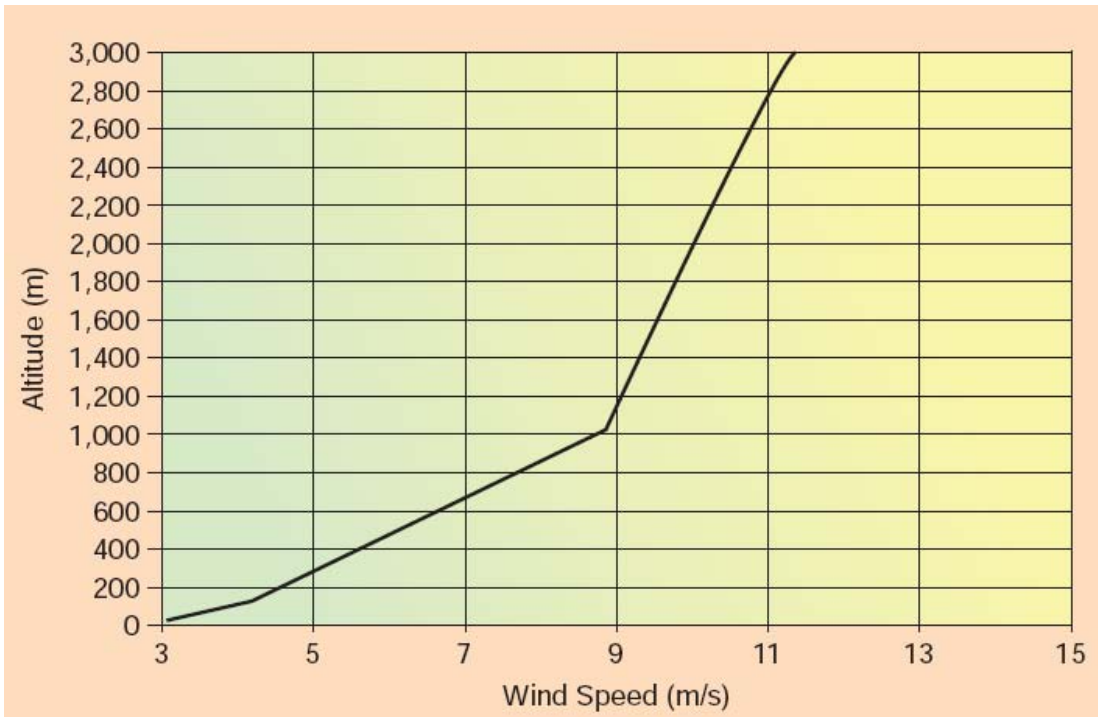
Figure 2. Wind-speed variation as a function of altitude; this data is based on the average European wind speed of 3 m/s at ground level 16
