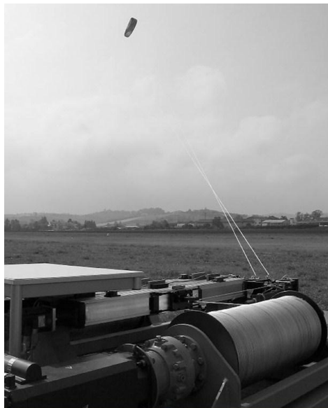
Figure 13. KE-yoyo small-scale prototype operating near Torino, Italy 9
