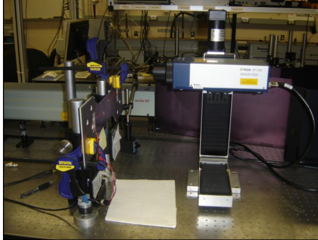
Figure 47: Laser Vibrometry Equipment
