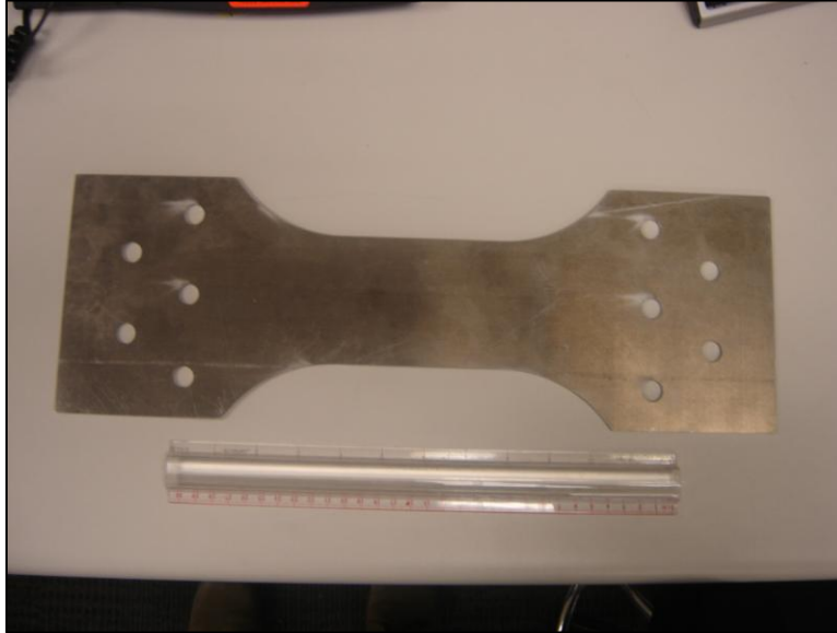
Figure 48: Aluminum Dog Bone Test Article
