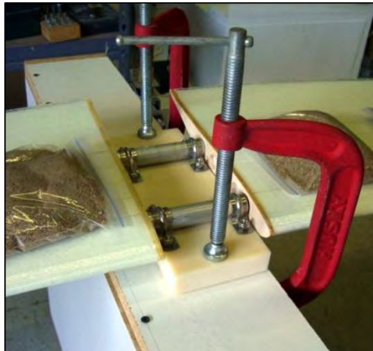
Figure 17: CLMax Wing Load Testing
