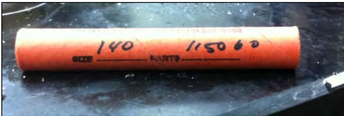
Figure 3.14. Starlite Bit Casing with Product Information
