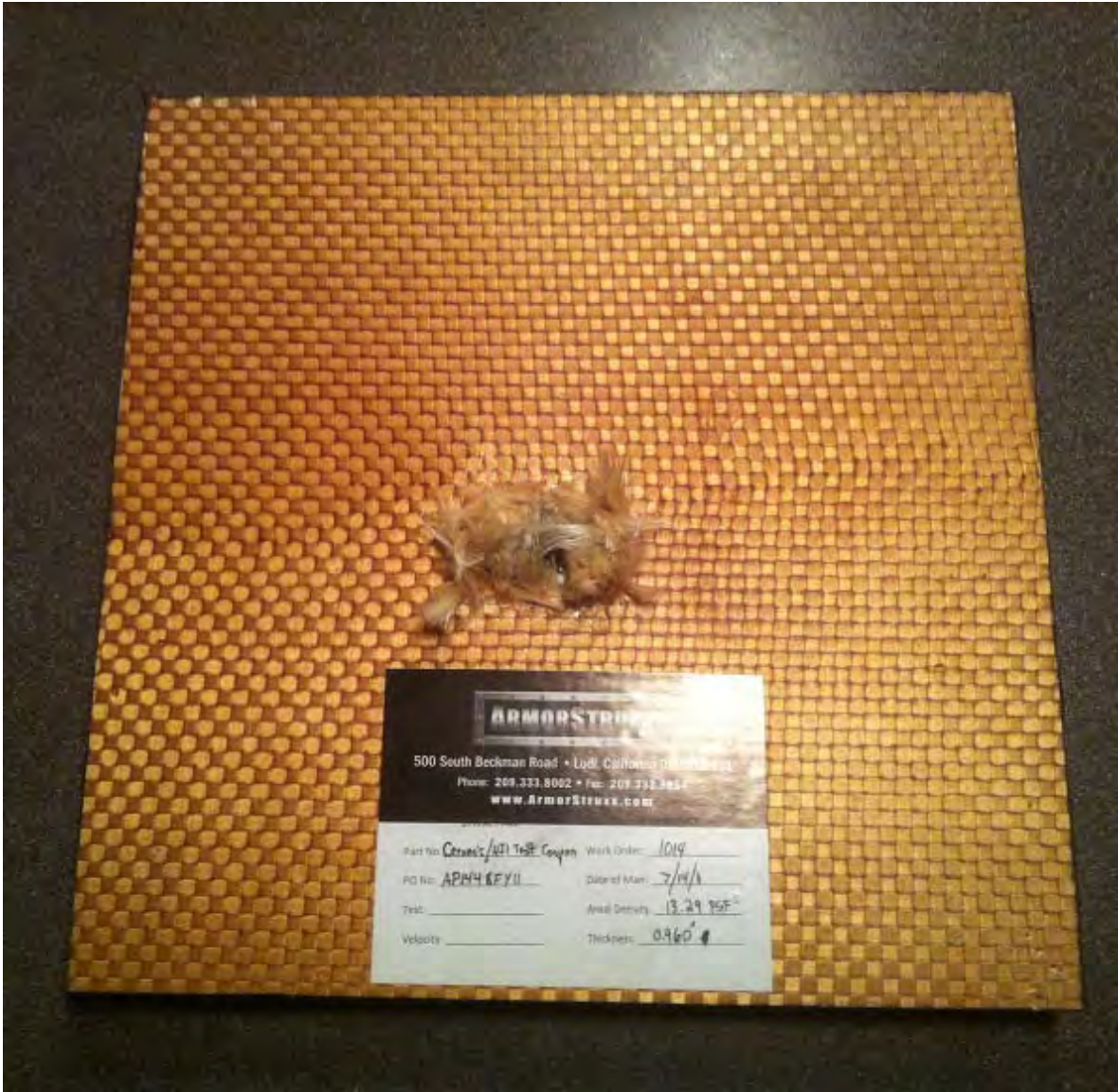
Figure 4.11. Successful Ballistic Test on the Two Layer Armor
