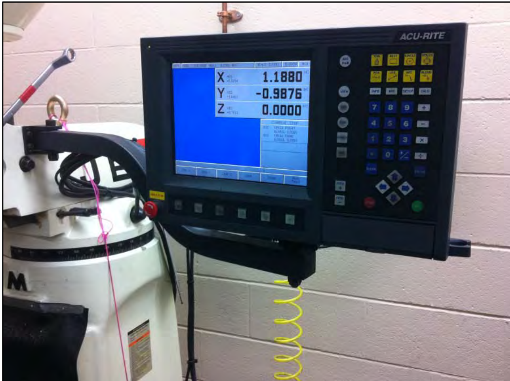
Figure 3.29. Acu-Rite Display Used to Control Location and Depth of the Drill Operation
