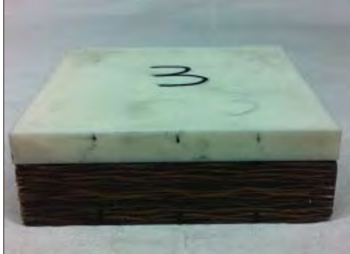
Figure 2.3. Two Layer Armor with Ceramic Frontal Plate and HJ1 Composite
