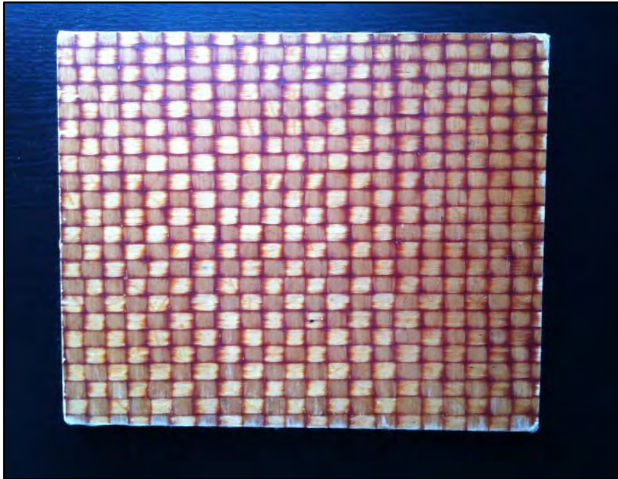
Figure 3.2. HJ1 Composite from ArmorStruxx
