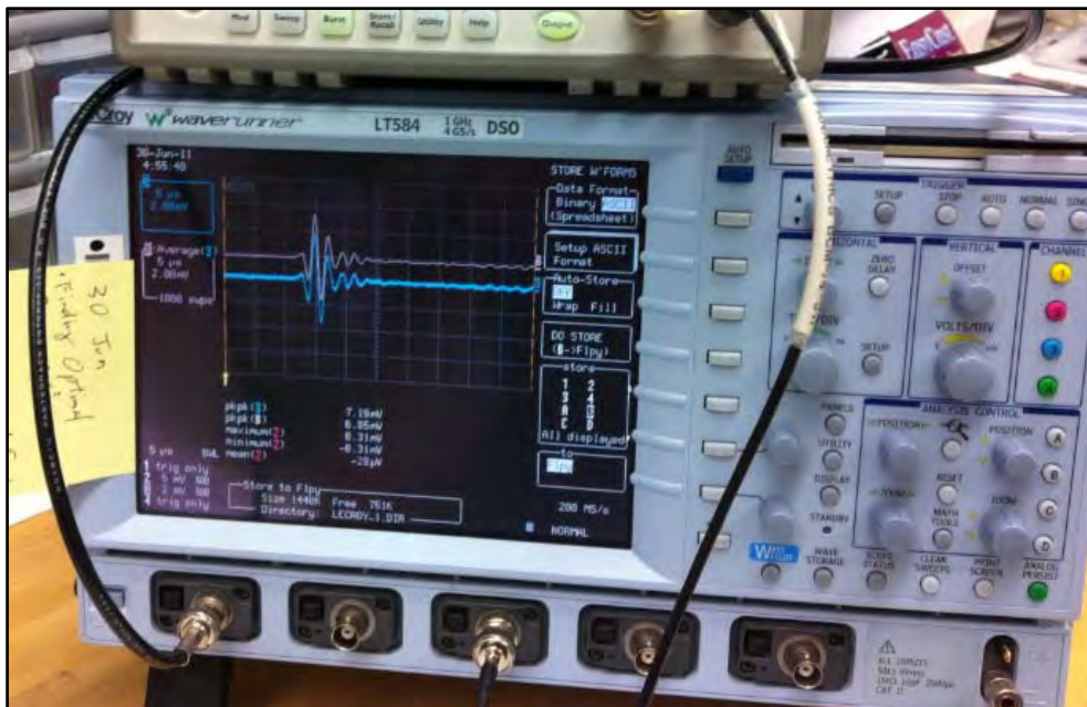
Figure 3.21. Oscilloscope Used to Capture Output Wave Propagations
