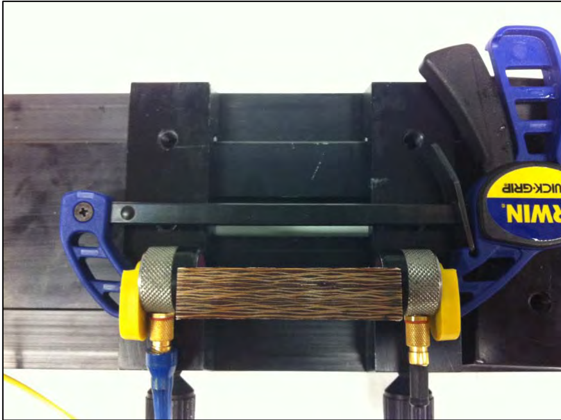
Figure 3.26. PZT Sensors Placed on the Composite in an Offset Orientation
