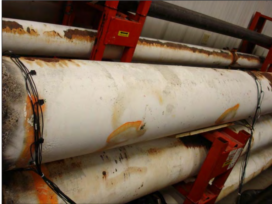
Figure 2.10. Photo Showing One Setup for Using CT Approach for Pipeline Health Monitoring (Royer, Velsor & Rose, 2009)
