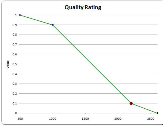
Figure 20. Quality Rating Piecewise Linear Single Dimensional Value Function
