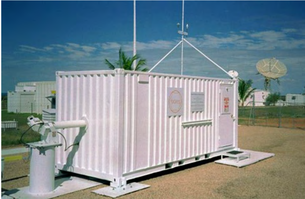
Figure 11. GONG observatory at Learmonth, Australia. The exterior portion of the telescope is noted on the near short side of the shelter. http://gong.nso.edu/instrument/
