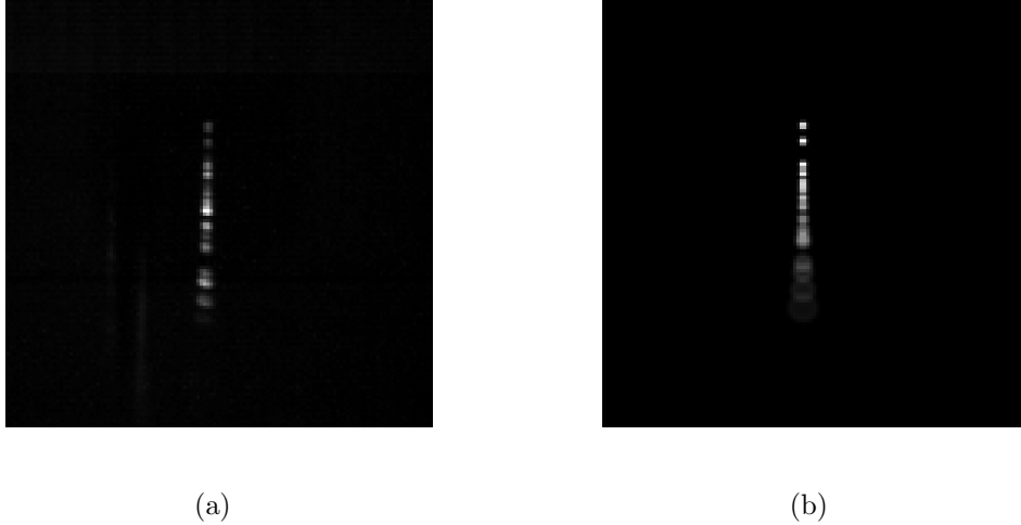
Figure 3.8. Measured and simulated, respectively, neon pen lamp data. The longer wavelengths are near the bottom of the images.
