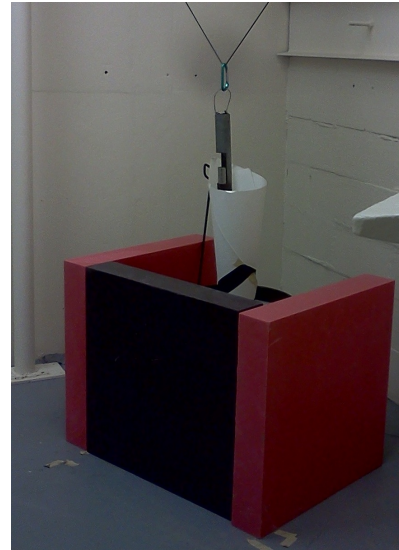
Figure 21. Picture of the source at the full height of the pulse. The funnel was made of poster board and was used to guide the source back into the container.
