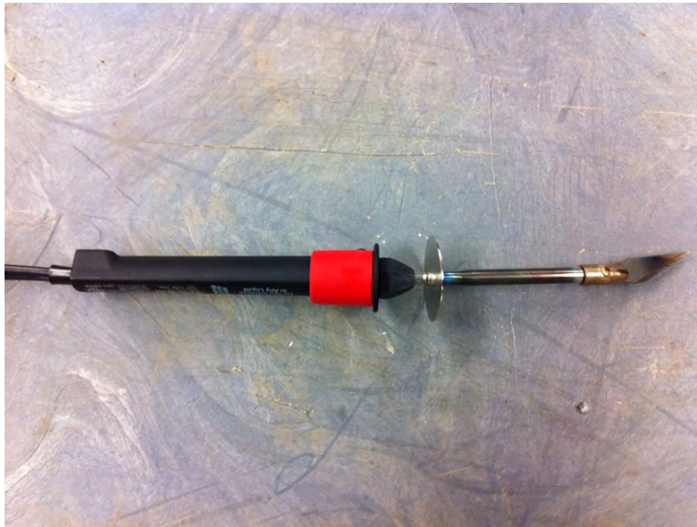
Figure 15. Hot knife used to cleave ends of the fibers used during this investigation. The blade is adapted to attach to the end of a standard electronics soldering iron.
