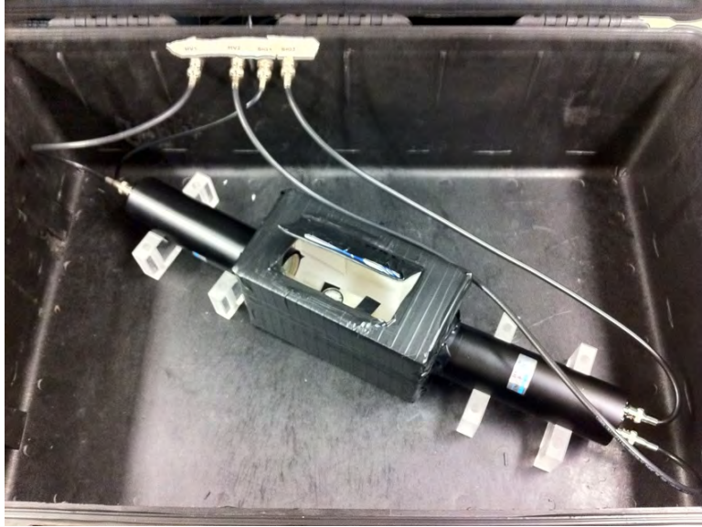
Figure 20. Image of the cardboard dark box. Electrical tape is triple-wrapped around all faces and edges of the box. Two holes are cut on opposite ends of the box to allow for insertion of the PMTs. A hatch is cut on the top of the box to allow for fiber bundle and radioactive source placement. The advantage of this design is it's darker than the larger plastic dark box used previously, while also being portable. The disadvantage of this design is the fragile nature of the tape adhesive. Changes in temperature made the tape peel off and loosen the PMTs from the box, resulting in fiber slipping.
