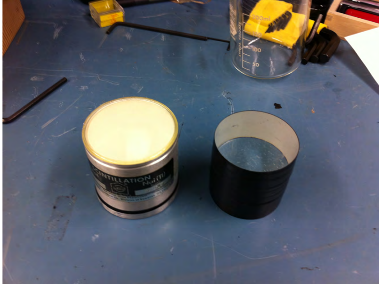
Figure 12. A picture of the bulk scintillator used during this investigation. The NaI scintillator is on the left and the BC-404 plastic scintillator is on the right. Electrical tape is wrapped around the plastic scintillator to prevent stray light from radially entering the scintillator medium. The end of the plastic scintillator not facing the PMT window is also blacked out for the same reason.
