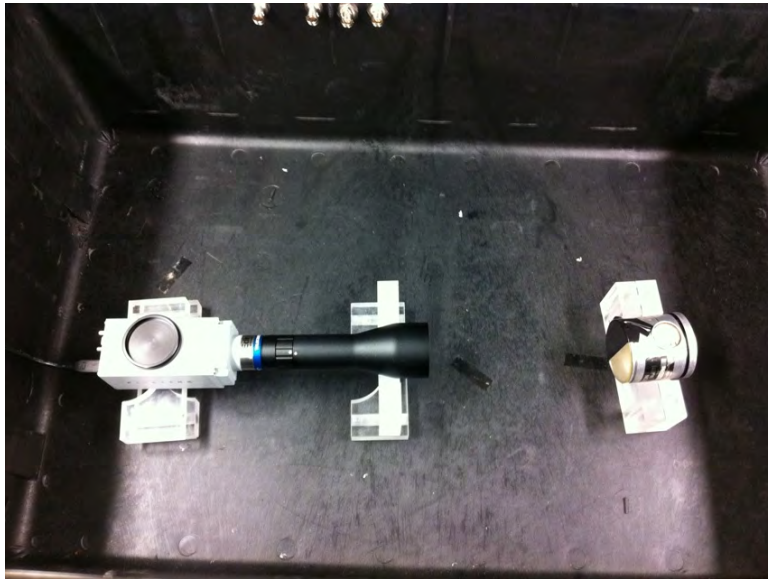
Figure 23. Experimental setup of NaI crystal imaging with the CCD camera inside the large dark box. The NaI crystal is placed at the focal length of the camera optics. Half of the crystal is covered with tape. The camera's FOV captures both the mask and the exposed crystal face. A Cs-137 source is placed on top of the crystal. Any scintillation light captured by the camera will only show up on the right side of image.
