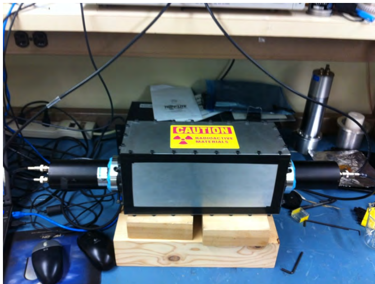
Figure 21. Full view of the aluminum dark box used for data collection during the dual-ended readout portion of this investigation. The PMTs are secured to the box with set screw after pinching the fiber bundle inside the box. The box is designed with portability in mind, being placed in front of radiation sources that are not found in the laboratory.
