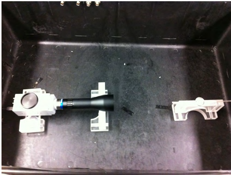
Figure 24. Experimental setup of 7x3 fiber bundle imaging with the CCD camera inside the large dark box. The closest fiber bundle face to the camera is located at the focal length of the camera optics. A Cs-137 source is placed on top of the bundle, centered along the length of the fibers.
