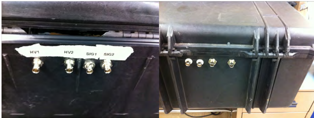
Figure 11. Left: Interior BNC connections for two pairs of PMTs. Right: Exterior BNC connections for the PMTs inside the dark box. These connections allowed for the PMT bias and signal cables to be connected while keeping the box completely closed and sealed.
