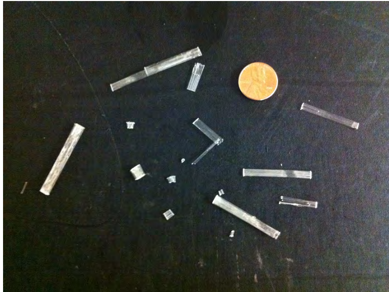
Figure 18. Fiber scraps from left from botched attempts at cleaving individual fibers, fiber ribbons, and fiber bundles. The fibers that were used for the fiber ribbon construction started out at 30 cm. When constructed the fiber ribbons ended up at 25 cm. The final bundle measured in at 19 cm. The difficulty in getting a clean fiber cleave resulted in wasting 33% of the initial fiber length.
