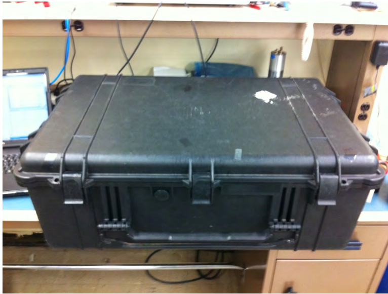
Figure 10. Image of the large dark box used for three experiments during this investigation. It is designed to be water tight. Water tight doesn't mean light tight, as discovered over the course of this research.
