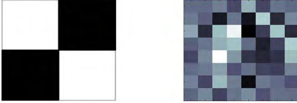
Figure 8. Difference between ideal image (left) and recovered image (right) in experimental results using the Moore-Penrose pseudoinverse.
