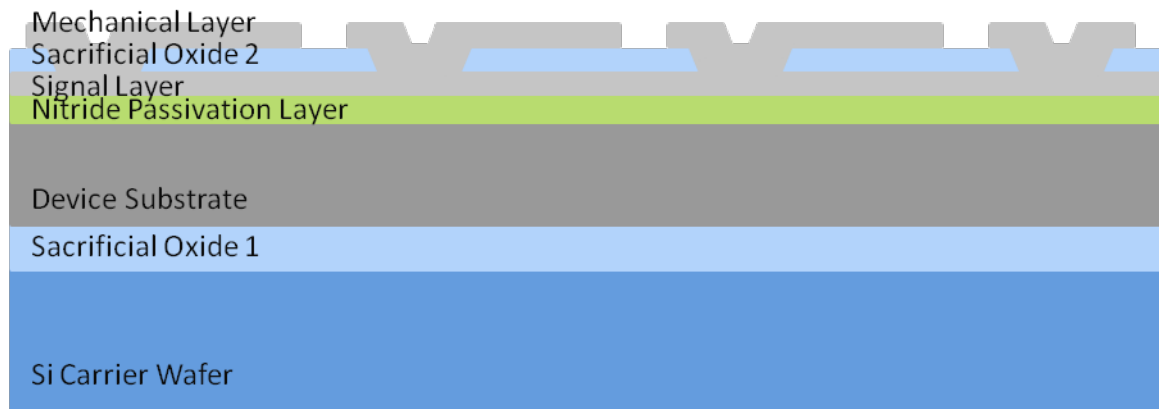
Figure 20 Silicon Carbide Process to Make the Strain Sensor
