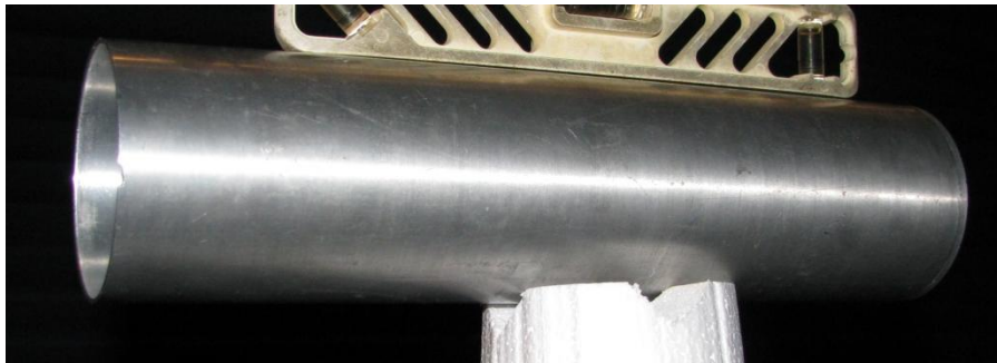
Figure 2: Cylinder with one end cap and one open end, “cavity”, on Styrofoam pylon
