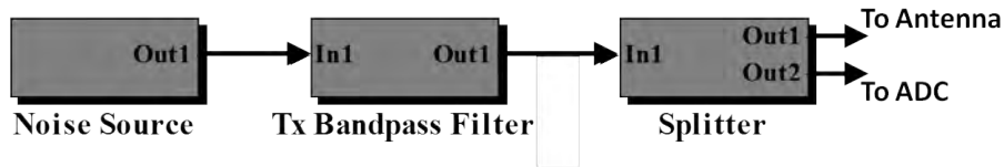
Figure 4.6. Components of the AFIT RNR transmit path as modeled in Simulink ® .
