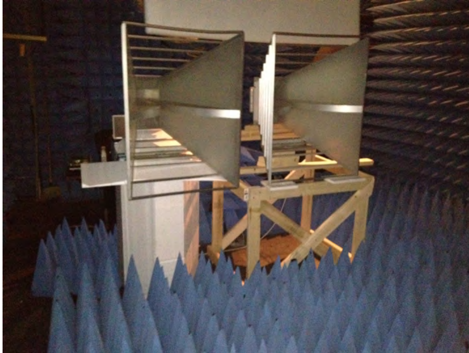
Figure 3.11. Two UHF standard gain horns are used in place of the LPAs to eliminate an unknown variable in the AFIT RNR model.
