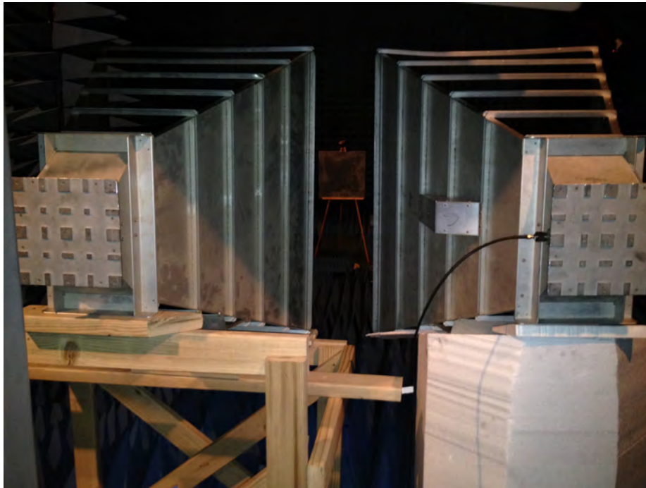
Figure 3.12. The 2 ft 2 flat-plate target located at a distance of 6 m from the RNR with two standard gain horns is shown.
