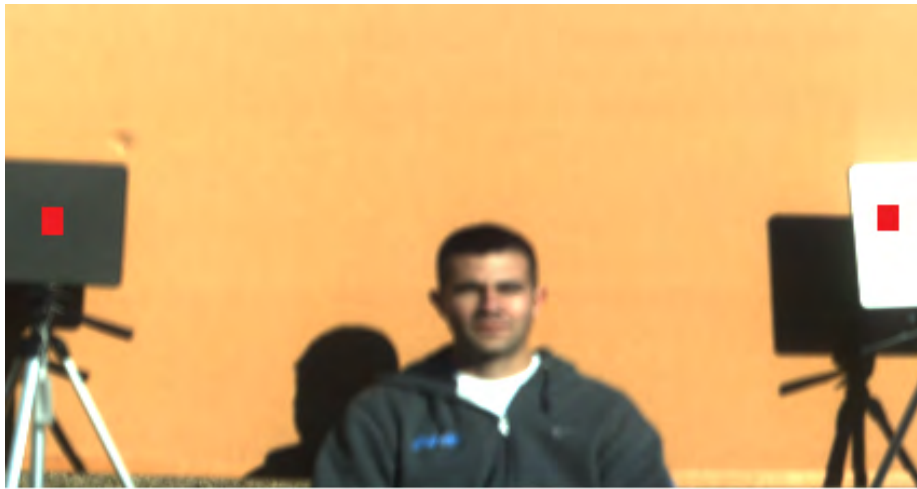
Figure 3.8: White and Gray reflector panels used for reflectance calculations (red squares).
