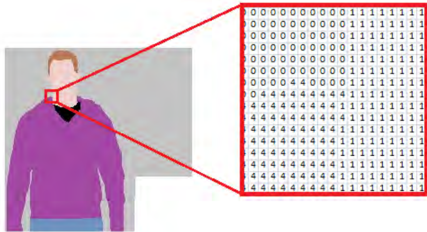
Figure 4.4: Pixel map to mimic image taken with PHIRST Light II camera. The pixel map is the result of clustering the scene image following AMG and morphological body outline and body composition by parts.
