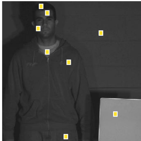
Figure 4.2: Location of signature acquisition points (yellow squares) for the two signature acquisition methods (spectroradiometer and hyperspectral camera).
