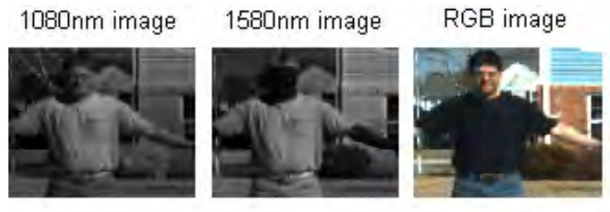
Figure 2.7: Original imagery from the 1080nm, 1580nm, and RGB cameras used for skin detection [16].
