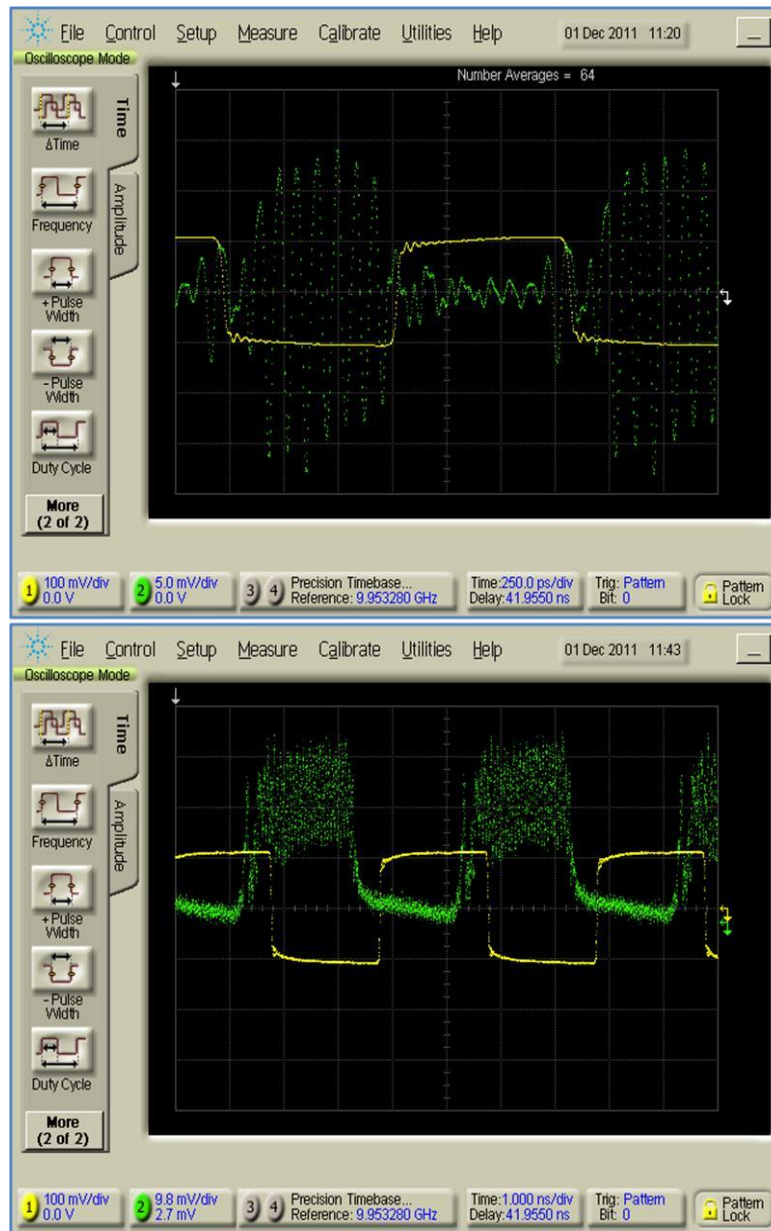
Figure 4.24: Two separate data signals over the same length of fiber experience the same time delay (41.9550 ns) appropriate for 8.566 m SMF at 1550 nm wavelength.
