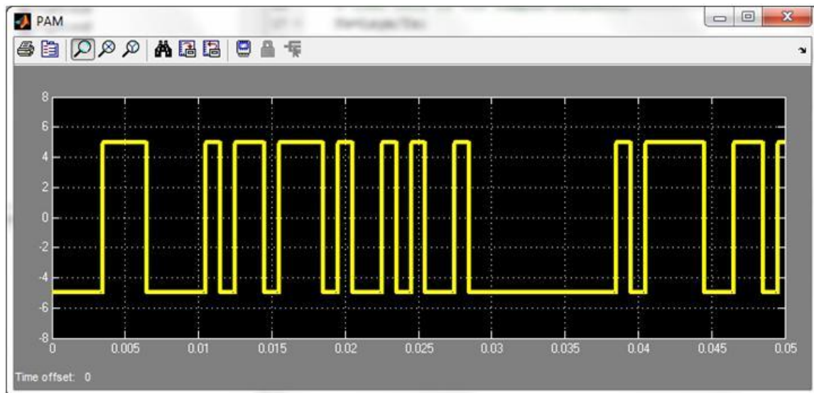
Figure 6.10: Output of a simulated binary rectangular polar PAM signal with A=5V and T_b=1 ms.
