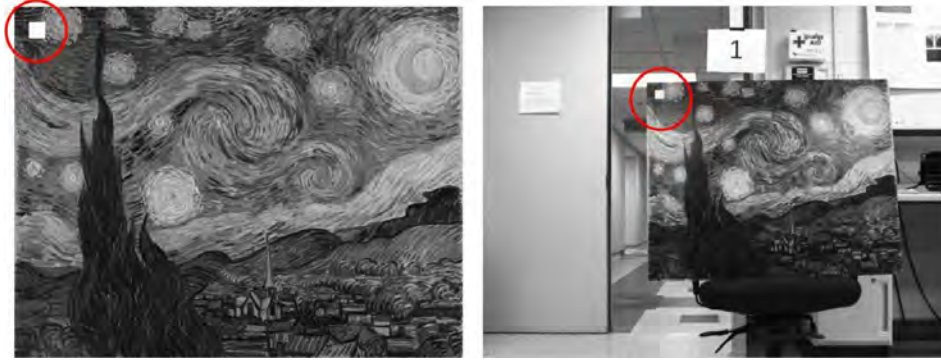
Figure 3.4: Pixel-to-board frame mapping. In order to convert digital cal -frame coordinates (pixels) to actual printed cal -frame coordinates (meters) for all automatic SIFT matches found, a transformation matrix is constructed by comparing the digital and printed cal -frame coordinates of four known points (corners of the white square).
