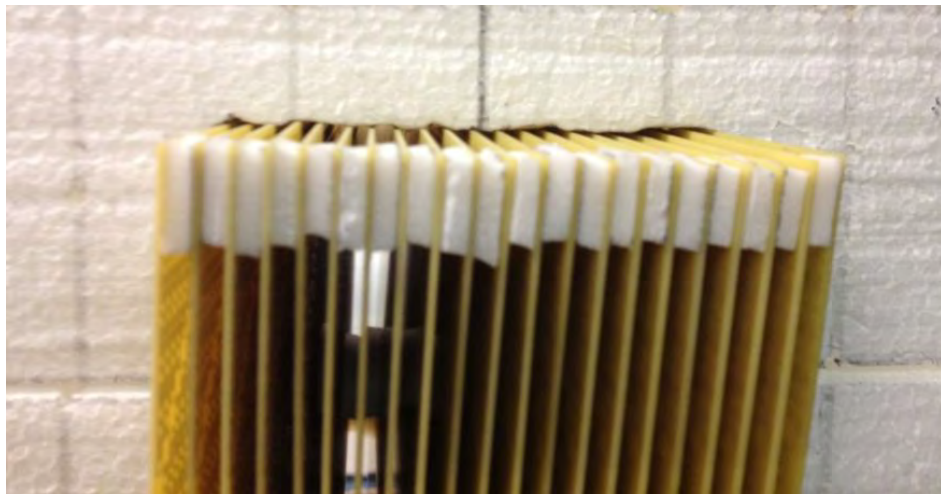
Figure 96. End view of the back, compression section of the field concentrator placed in the foam holder. As with the angled side view of the loaded target, some uneven back edges exist. This view also allows one to see uneven spacing in the board separation. The uneven spacing is due to the uneven Styrofoam on which the boards are sitting.
