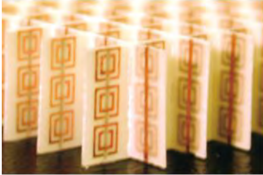
Figure 35. LHM sample built and tested in [57]. The sample was built as a periodic array of SRRs and wires and was designed to resonate at 10.5 GHz.
