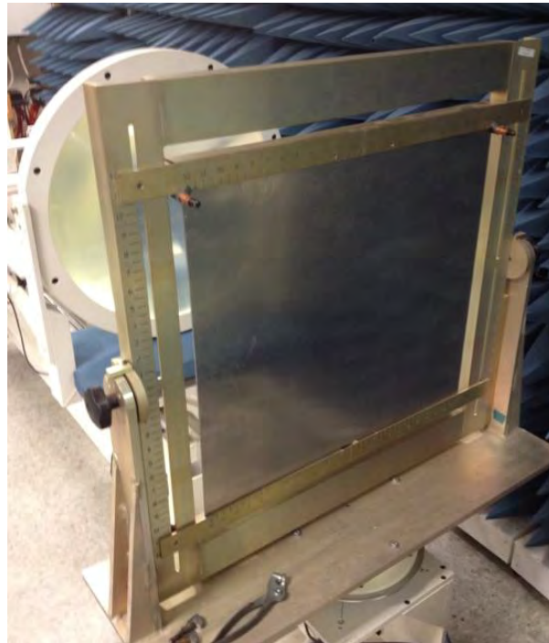
Figure 88. Metal plate held in the center mount. The metal plate was used to find the location of the zero phase plane in the time domain so that the NWA gating window could be set to include the target.
