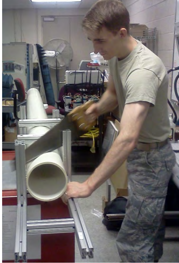
Figure 39: Machining PVC Pipe for PPWG Rolled-Edge Frame
