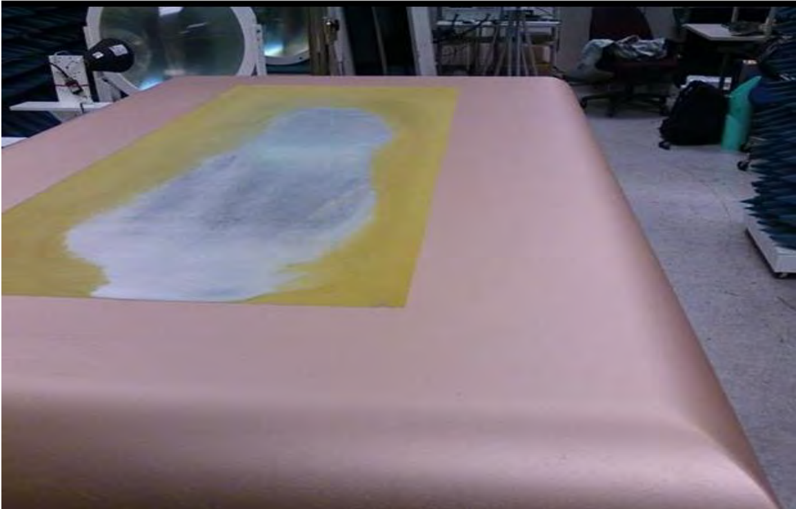
Figure 47: Top Plate Under Repair to Remove Excess Primer
