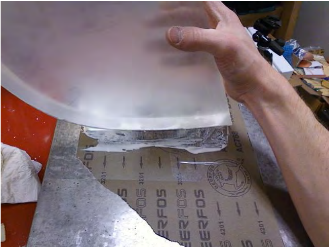
Figure 65: Polishing Lens With Compound
