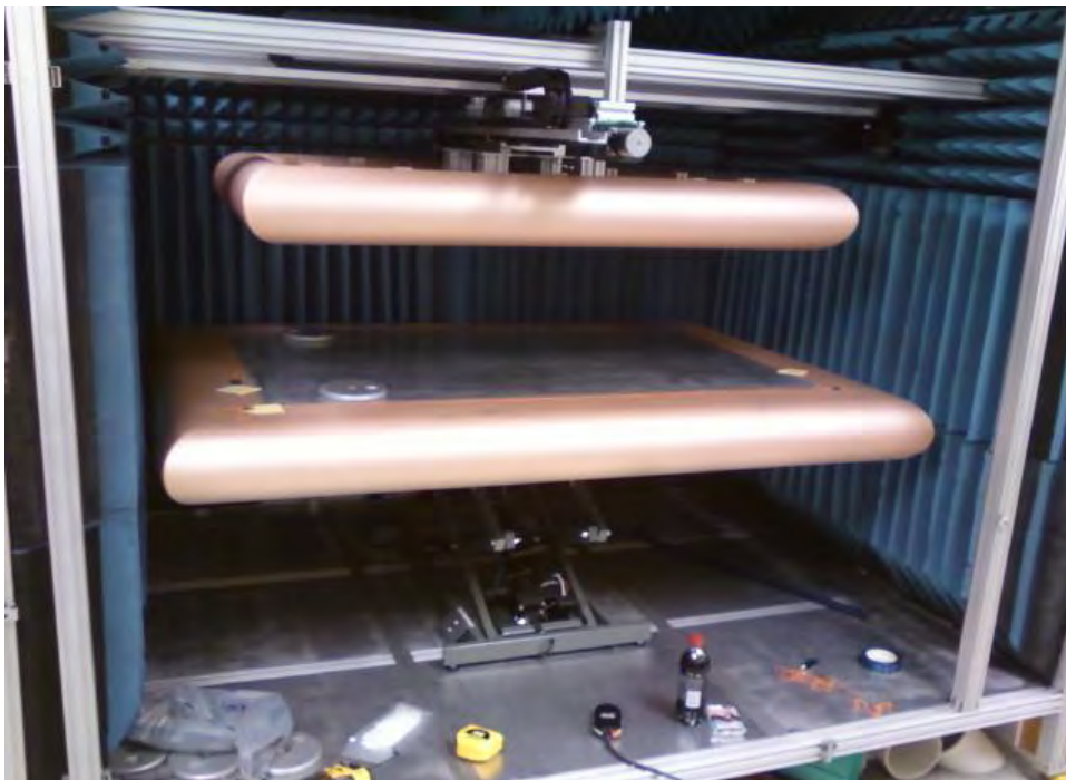
Figure 57: General Positioning of Scissor Lift and Bottom Plate
