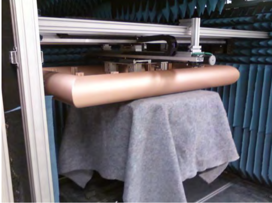
Figure 54: Using Lift to Install Top Plate (Raised)
