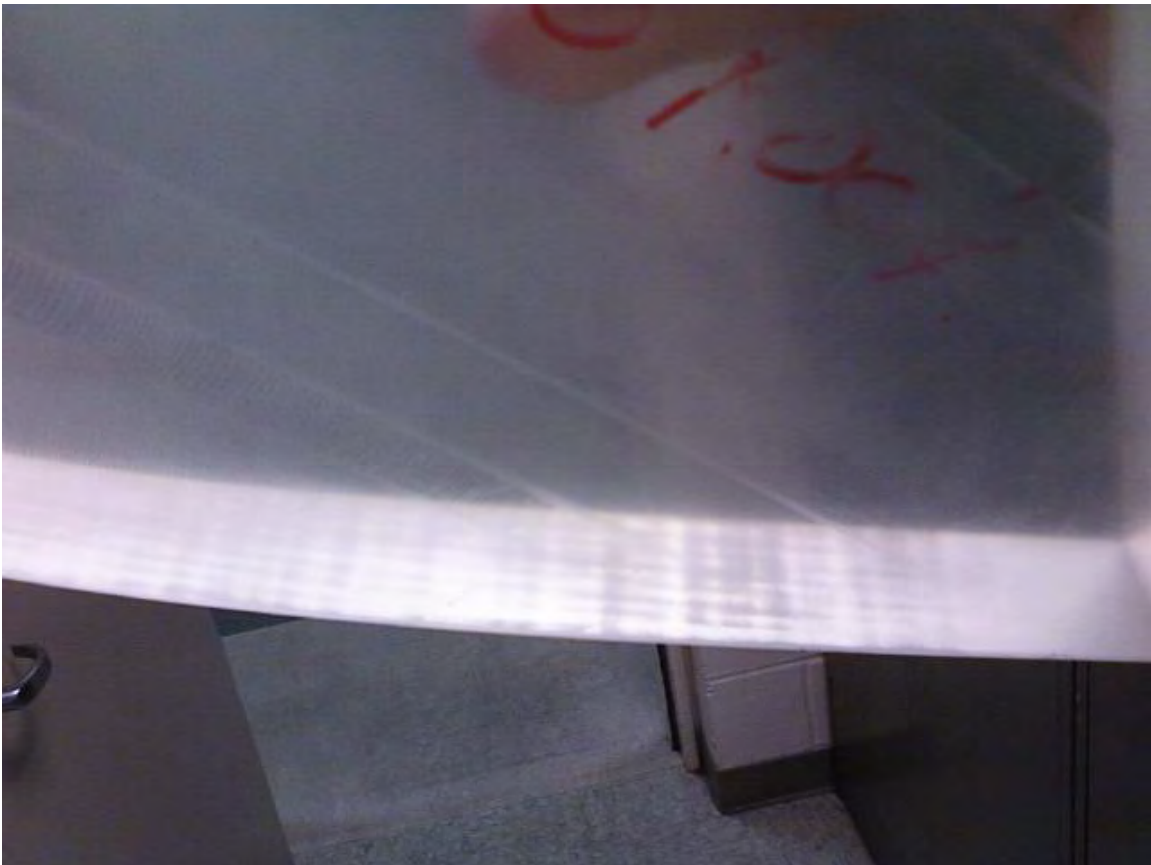
Figure 64: Bright Machine Marks in Profile Surface of Lens
