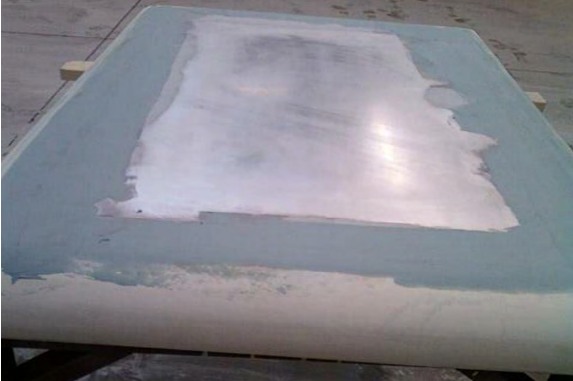
Figure 44: Top Plate with Light-Weight Filler Applied
