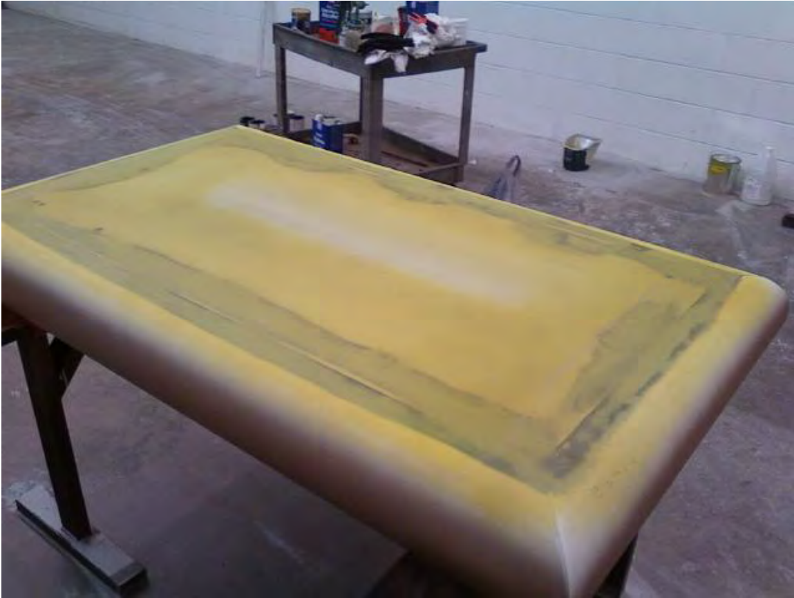
Figure 45: Top Plate with Primer Applied
