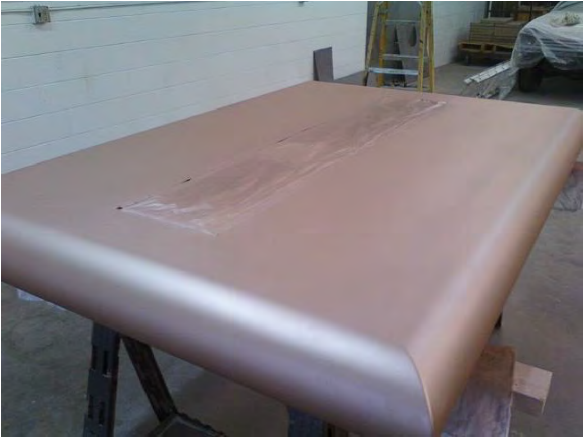
Figure 46: Bottom Plate with Two Conductive Coats and Clear Top Coat Applied
