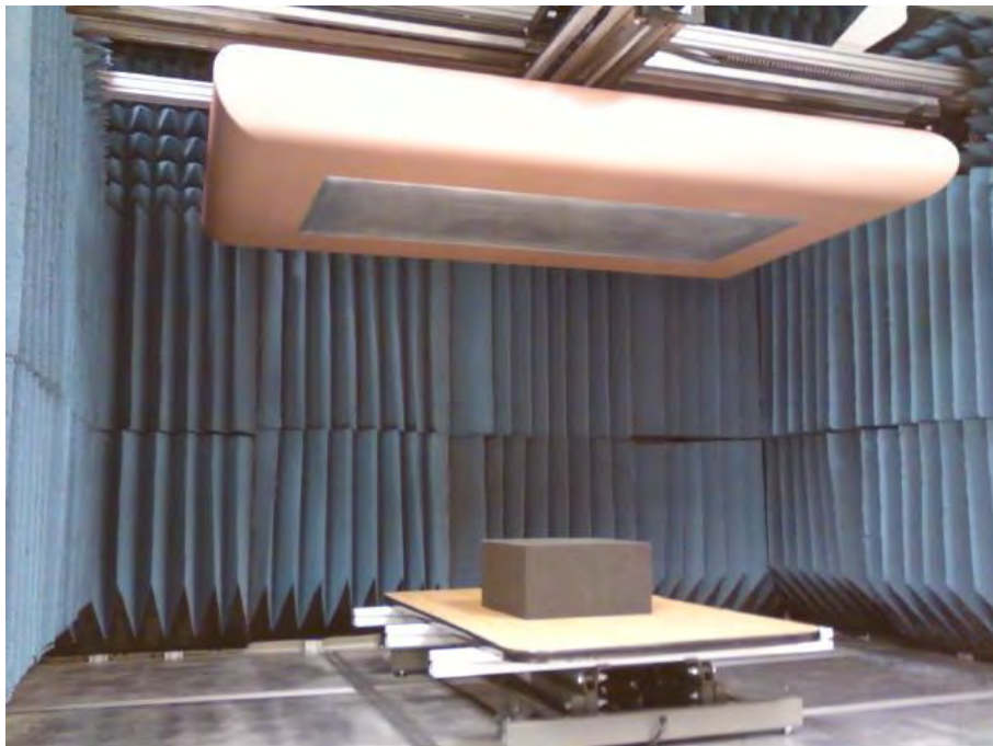
Figure 55: Using Lift to Install Top Plate (Lowered)
