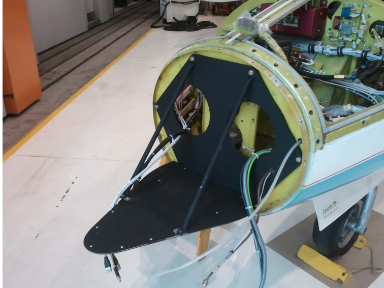
Figure 4.3: Mounting plate in nose cone of Learjet.
