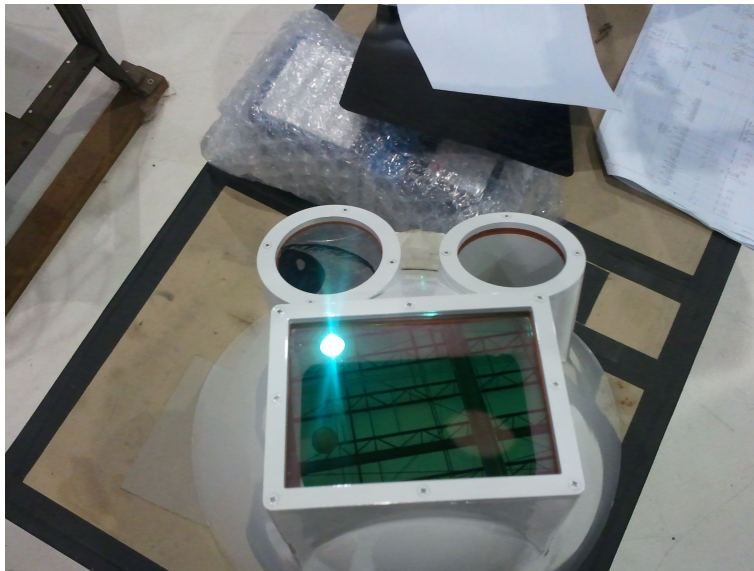
Figure 4.1: Nose cone of Learjet modified with panes of glass to allow sensors to see through nose cone.
