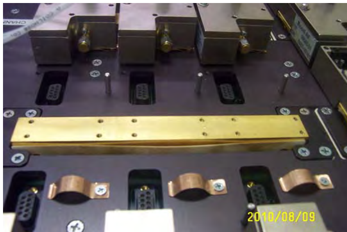
Figure 57. Heater bar for three test modules
