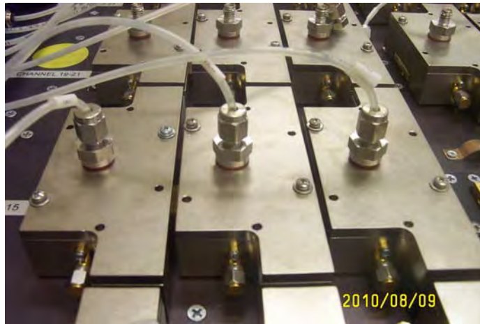
Figure 59. Test module covers and nitrogen tubes attached
