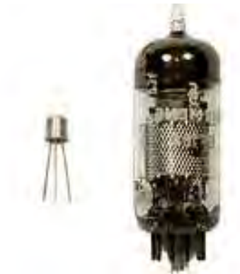
Figure 1. Relative size comparison of a transistor (left) and a vacuum tube (Nobelprize.org, 2010)
