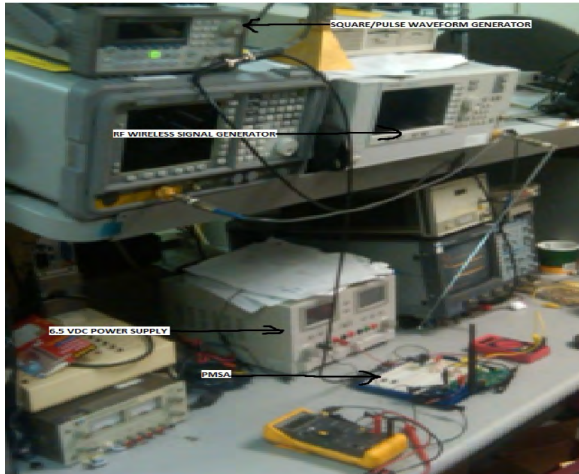
Figure 3.7: PMSA test bed
