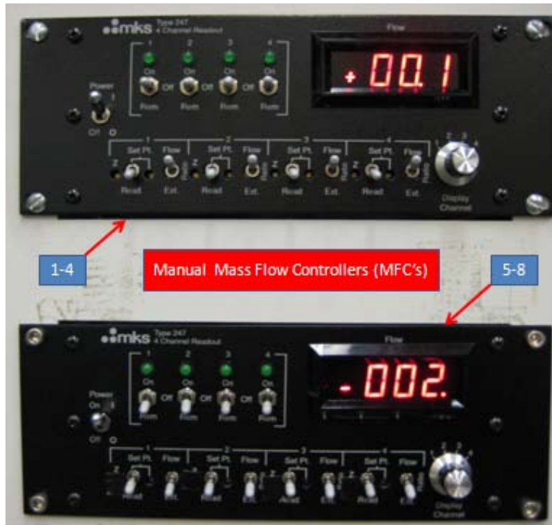
Figure A.2: MKS Manual Mass Flow Controllers (MFC's): switches 1-4 on the top MFC and channels 5-8 on the bottom MFC
