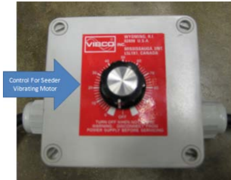
Figure A.10: Control knob for one of the two vibrating motors attached to the seeders
