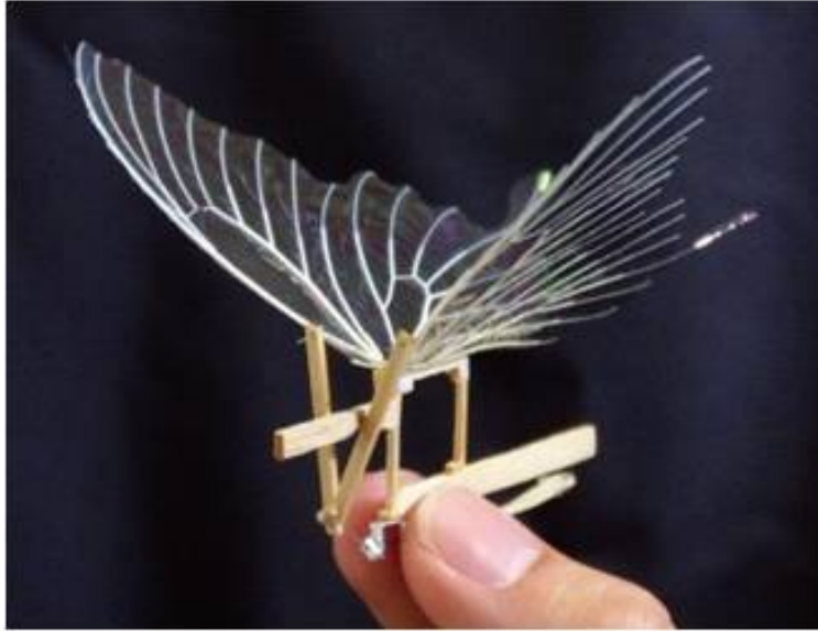
Figure 24: Tailless Ornithopter Mimicking a Swallowtail Butterfly [92]
