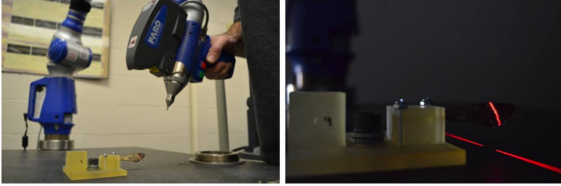
Figure 43: Faro Laser Line Scanner Actively Scanning Wing
