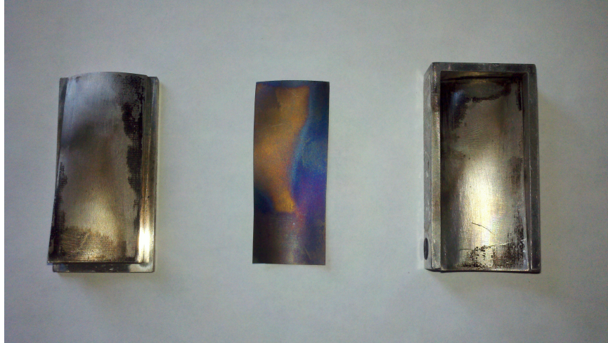
Figure 54: Machined Aluminum Mold with Sample Nitinol Sheet
