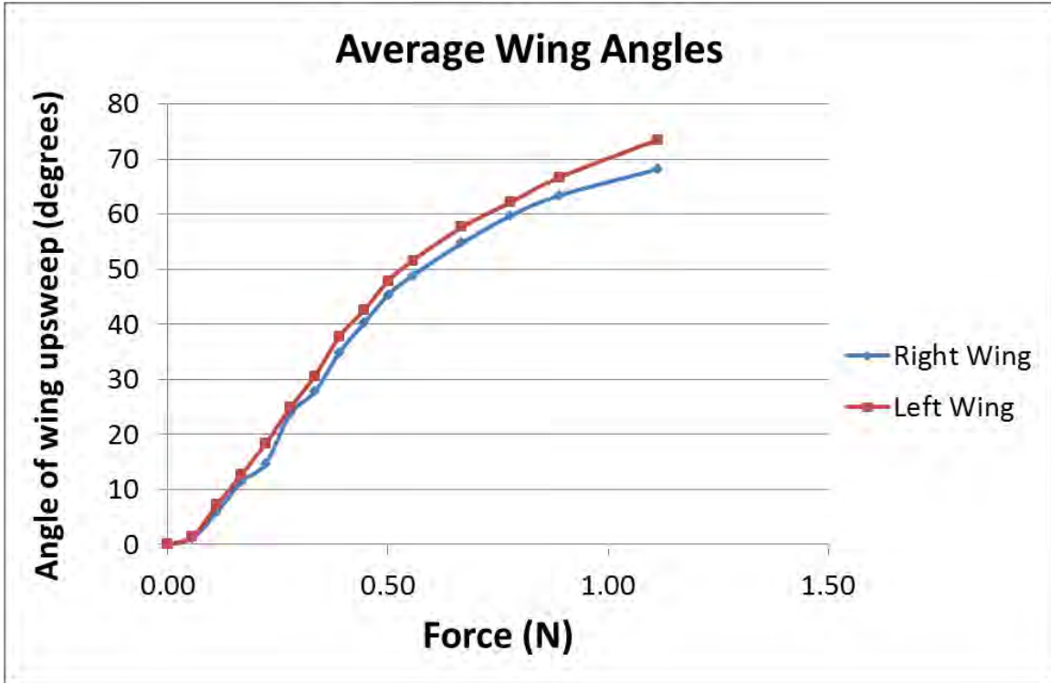
Figure 95 - Average wing angle for right and left wings for the first iteration
