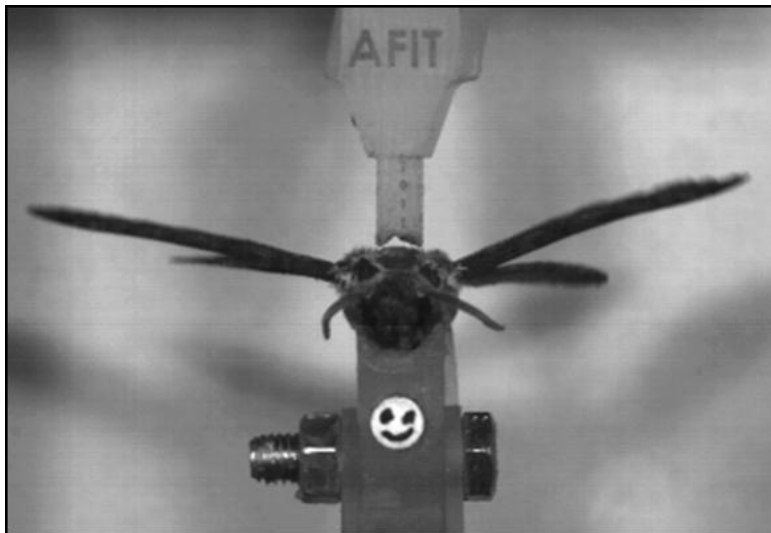
Figure 54 - Typical gap between tergum and push rod at bottom of vertical displacement cycle
