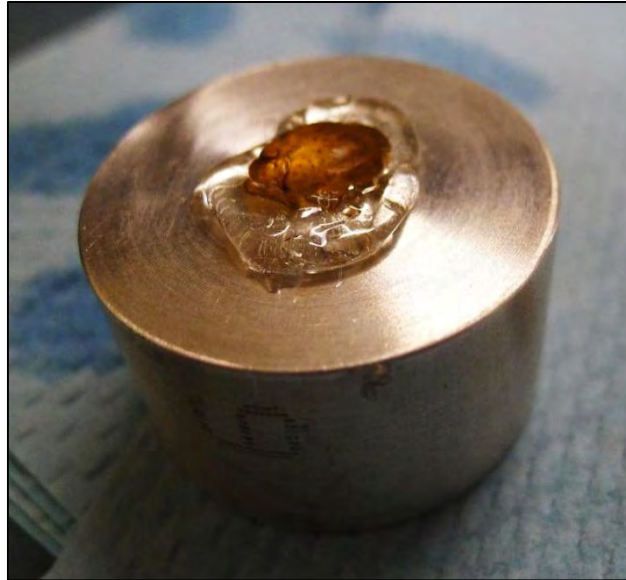
Figure 71 - Tergum mounted to puck with Crystalbond Hot Melt. The thermoplastic polymer completely fills and supports the cavity created by the removal of the flight muscles. The tergum is thin enough for light to pass through, giving the specimen the appearance of amber.
