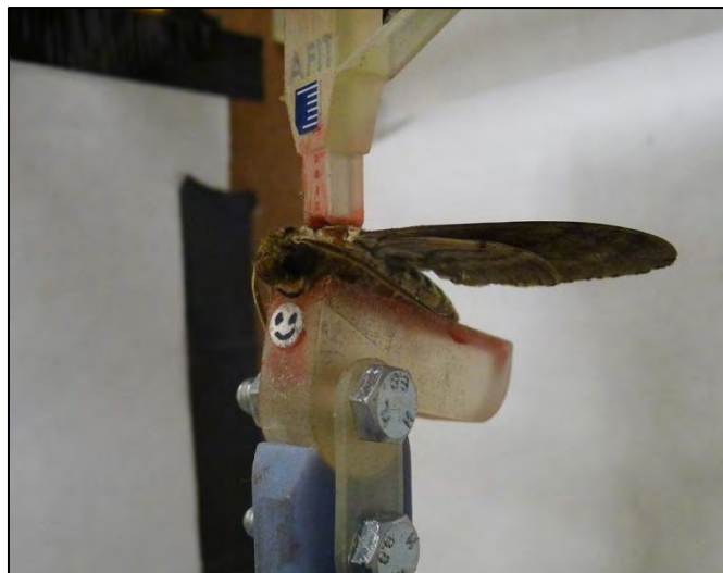
Figure 57 - Mounted specimen. Note the red wax above and below the moth. The “happy face” was used track the vertical displacement. The blue rectangle with white lines is a piece of a metric ruler with mm markings, used for determining pixels to mm conversion factors.
