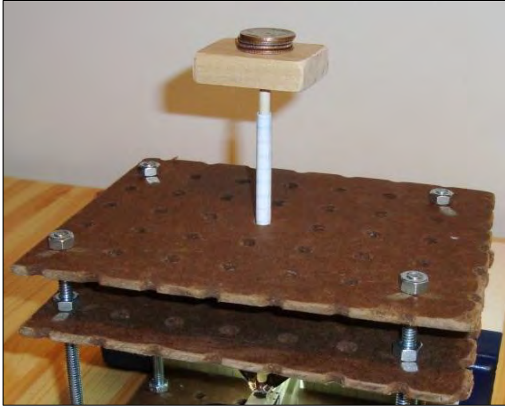
Figure 37 - Stack of quarters on push rod weight platform
