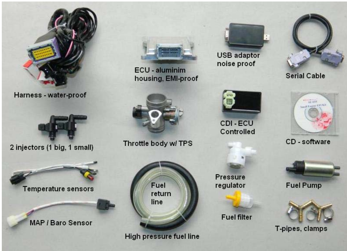
Figure 30: Ecotrons sourced fuel injection system as received from the company (Supplied by 24)
