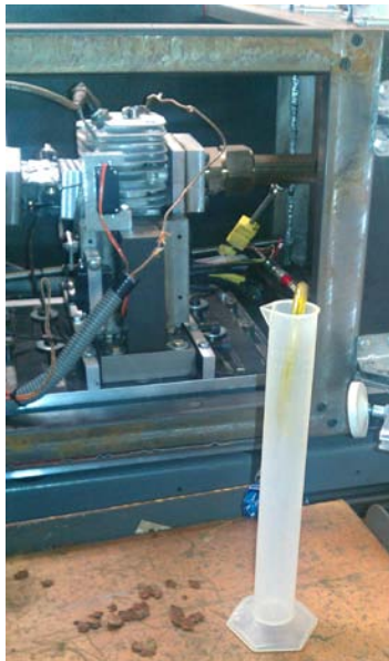
Figure 27: Fuel line and graduated cylinder used for fuel flow meter calibration
