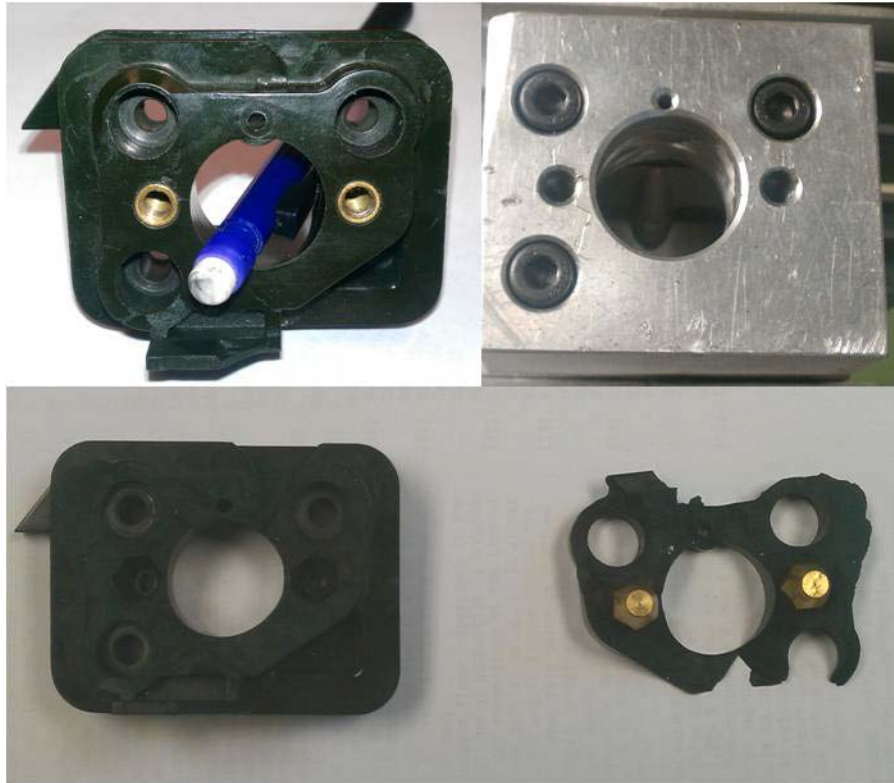
Figure 28: Top left is original spacer, top right is new aluminum spacer, and bottom is broken spacer
