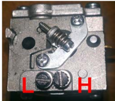
Figure 29: Walbro SDC 80 with low(L) and high (H) speed needles identified. Left side faces the engine and right side faces the inlet manifold
