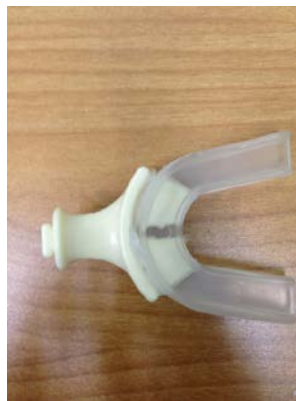
Figure 11. Custom Mouthguard with Accelerometer Mount
