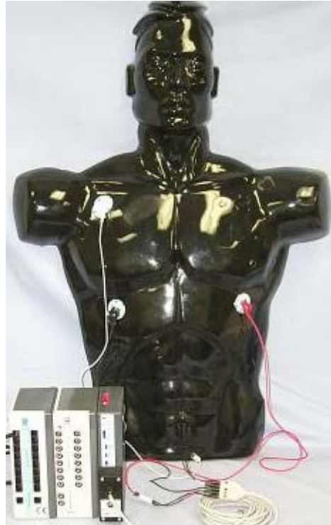
Figure 3: Electrode placement for ECG
