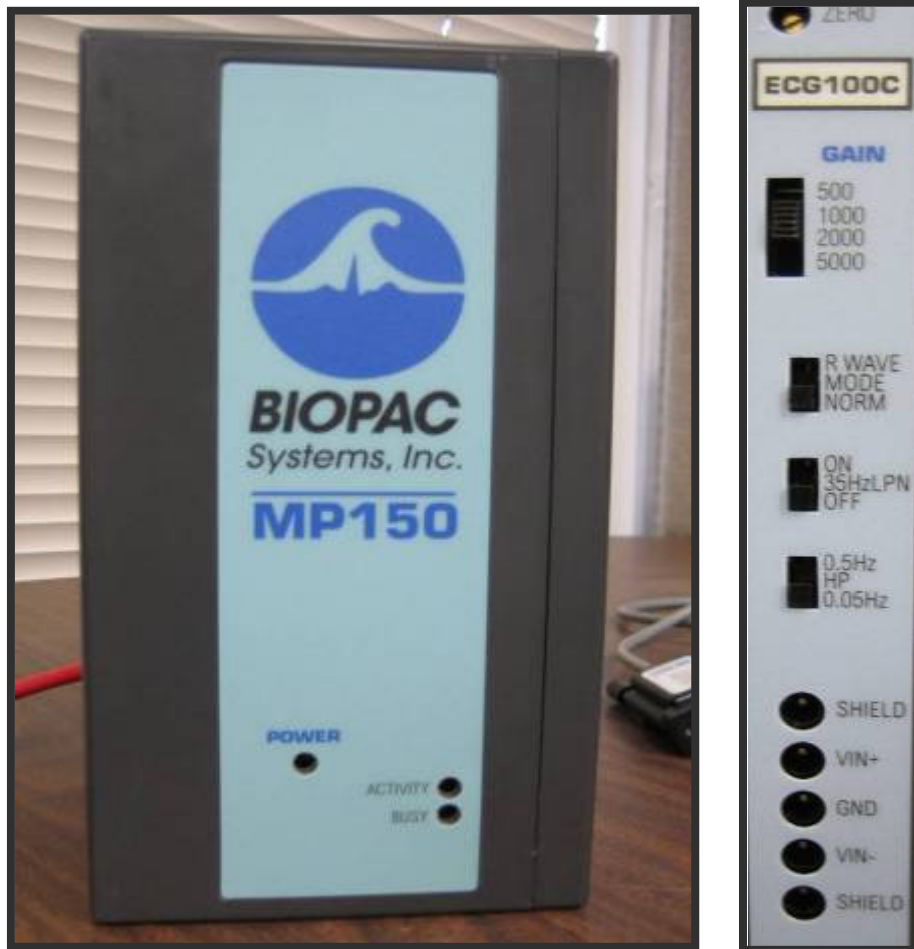
Figure 4: BIOPAC MP150 and ECG100C Amplifier
