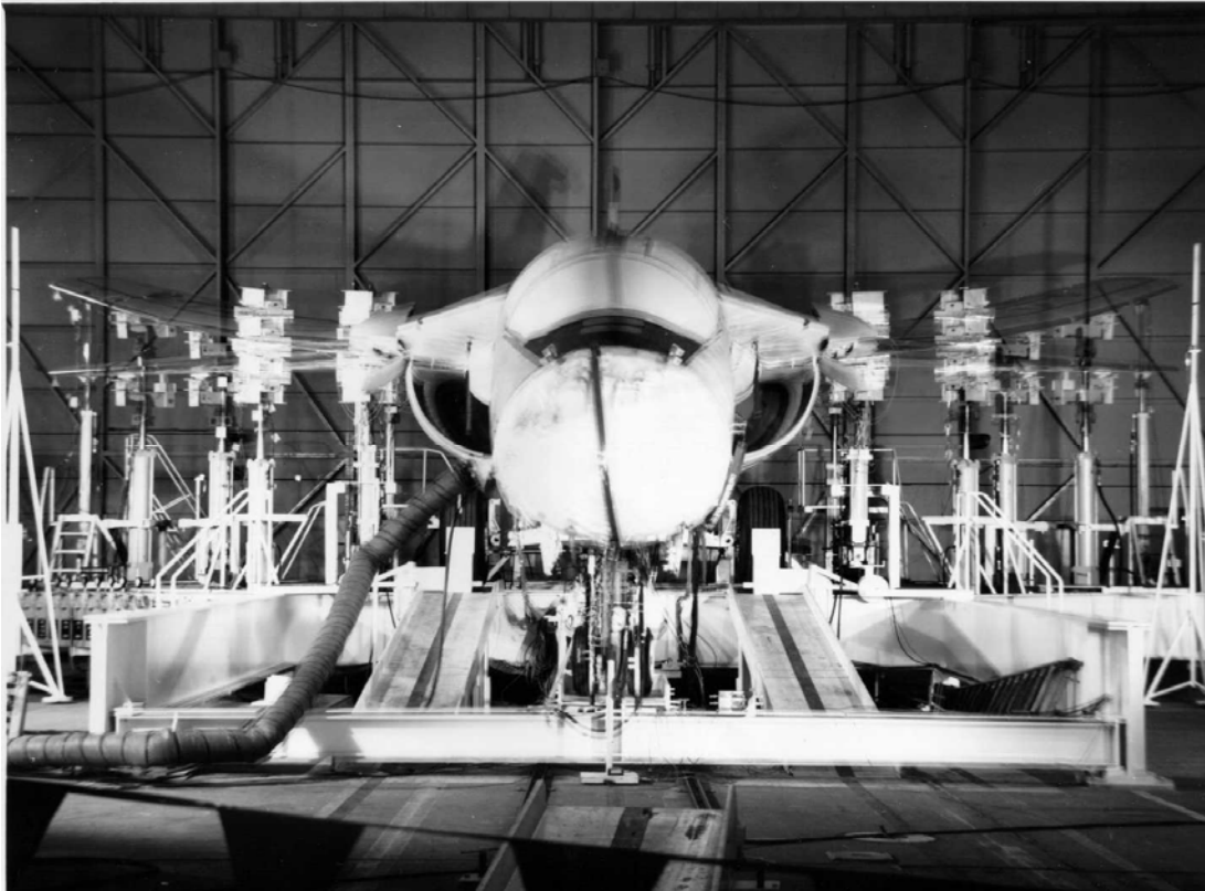
Figure 3-11. F-111 Cold Proof Load Test
