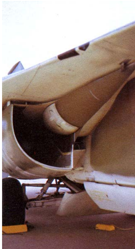
Figure A7-6. Triple Plow II – Note Wider Distance from Fuselage, No Splitter Plate
