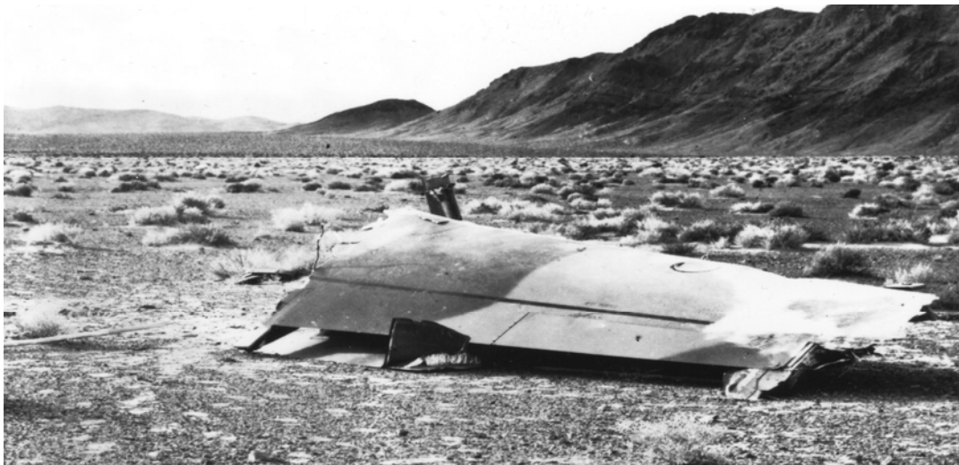
Figure 3-10. F-111A Wing Failure Dec 1969
