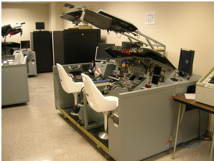
Figure 7. Cockpit Familiarization Trainer (CFT). 8
