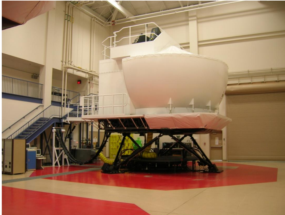
Figure 5. KC-135 OFT with Six Degree of Freedom Motion Base. 6
