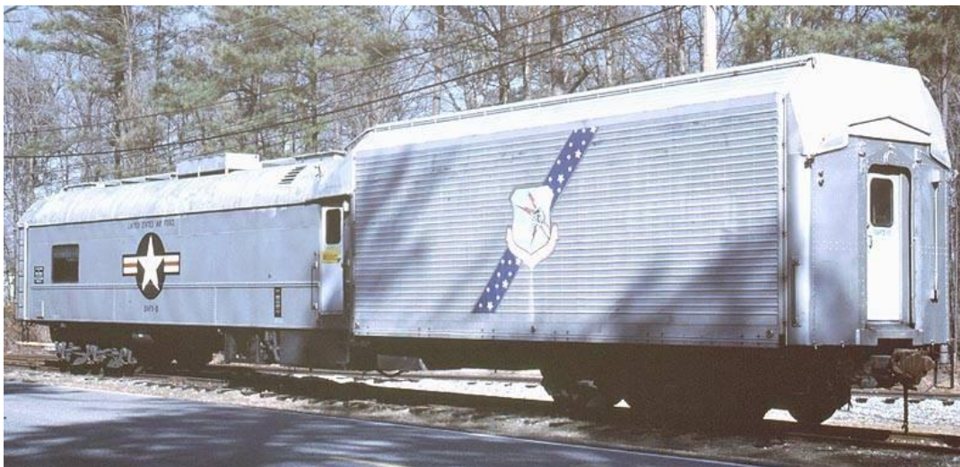
Figure 4. KC-135A Instrument Flight Trainer Railroad Car. 3
