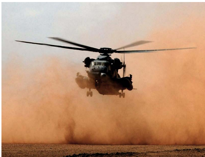
Figure 24. Onset of Rotary-Wing Brownout conditions
